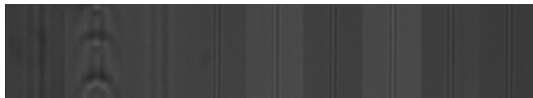
Figure 9: Typical microscope images of the structures inscribed at varying energy, constant speed and depth by 800nm high-repetition system.
