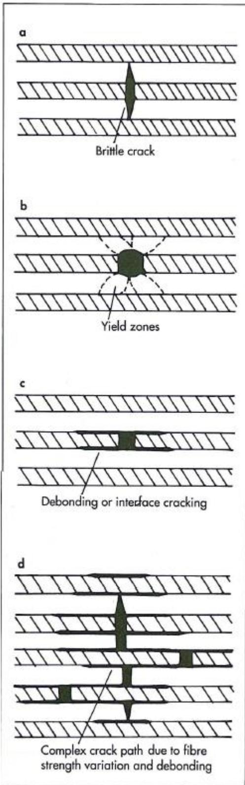
Fig.1 Fibre failure propagation<sup>4,5</sup>: a brittle cracking of matrix (high interfacial strength), b shear yielding of matrix, c interfacial failure, d propagation of fracture involving a and c.
