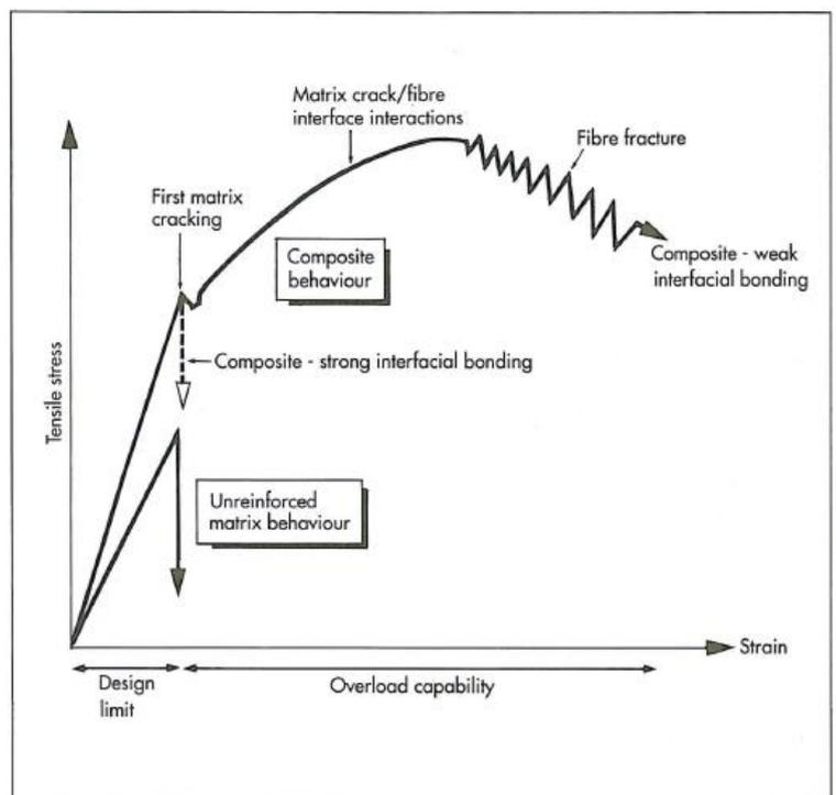
Fig 14 Continuous fibre reinforcement promotes 'graceful' or gradual Failure in ceramic matrix composites<sup>19</sup>. Three important elements of the failure process are labelled: matrix cracking, interfacial failure and fibre fracture
