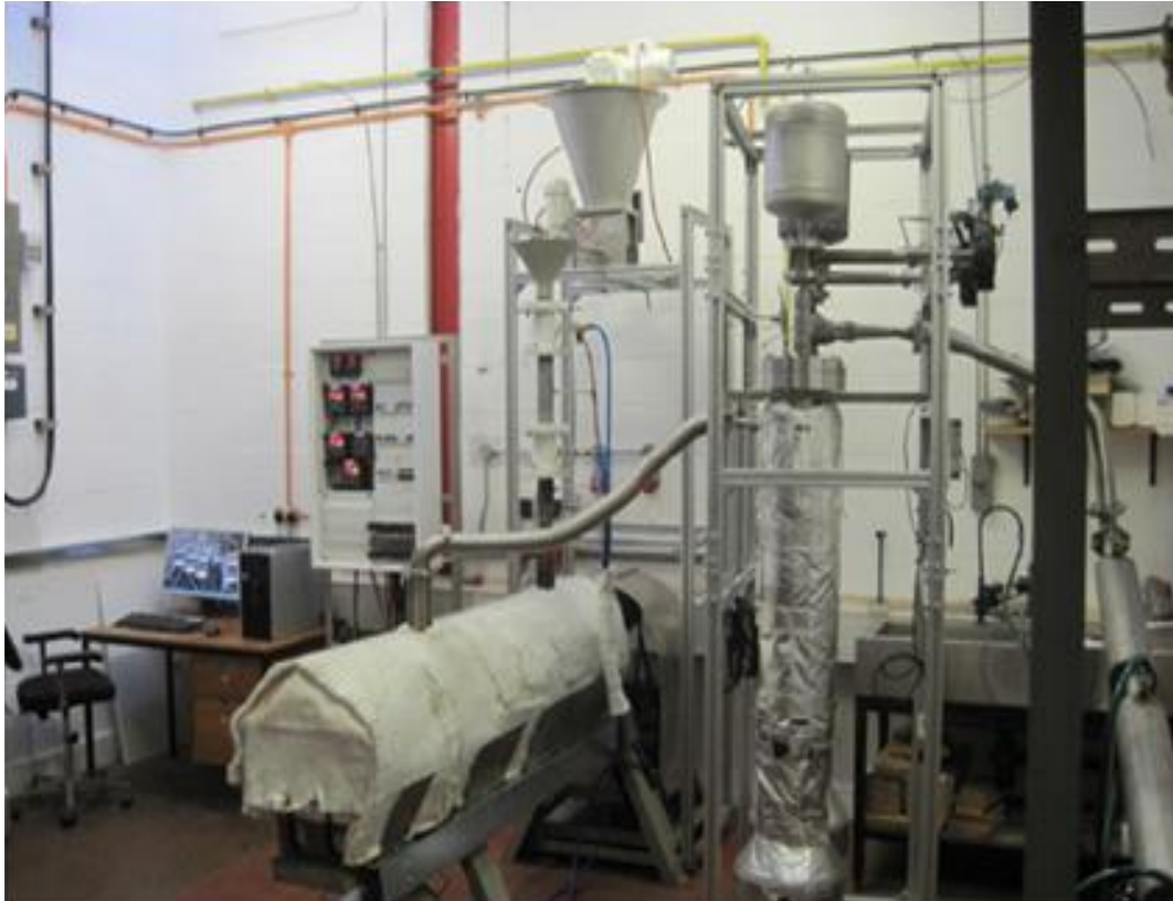
Figure 2 Pyroformer intermediate pyrolysis system Aston University
