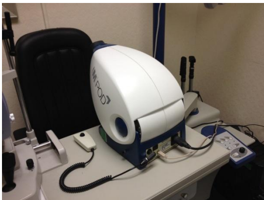
Figure 3.1: The MPS instrument used for this research project in position. The patient response button is to the left.
