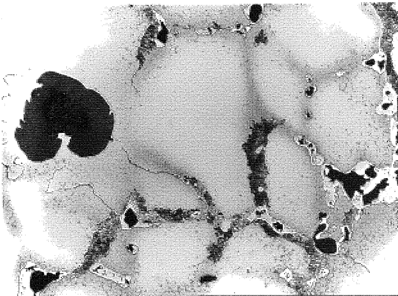
FIG. 51 Centre of 12 in section of 0.5 per cent manganese austenitic iron showing bainite near cell boundary carbides. Etched in 5% Nital x 100
