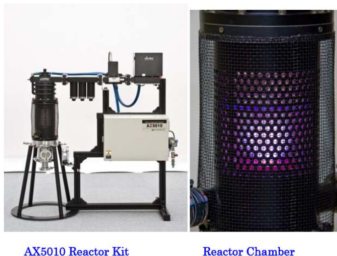
Figure 3.2 Left: 1.5 kW ASTeX™ MPECVD system in Aston University (Seki Technotron Corp.); Right: the reactor chamber with plasma inside.
