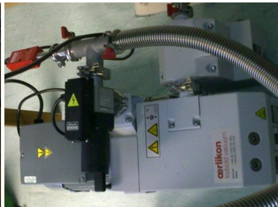
Fig.8 main rotary fan pump
