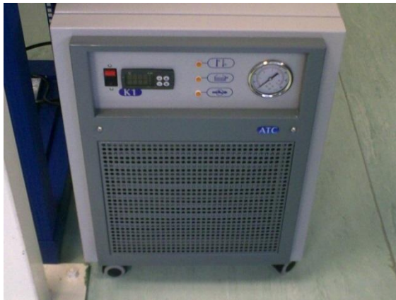
Fig.9 cyclic water cooling system
