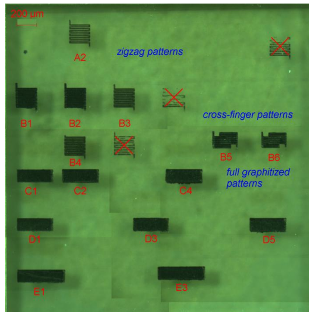
Figure 5.3 Overview optical image of micro-channel structures fabricated on single crystalline diamond substrate. Each pattern was processed using different parameters.
