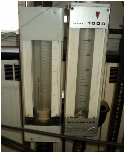
Fig. 2.4 . The two rotameters supplying air to the CFB system.
