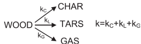
Fig. 4.4 . One-component mechanism of primary wood pyrolysis proposed by Shafizadeh and Chin (1977).
