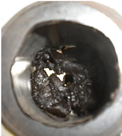
Figure 129: Mud-like paste in the bottom of feeder
