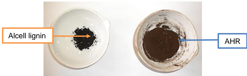
Figure 32: Alcell lignin and AHR after melt test at 200°C
