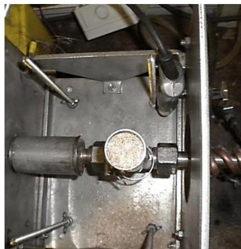
Figure 65: Feed backing up in the vertical feeding tube between the metering screw and the high speed feed screw in test 8.
