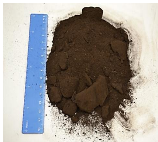
Figure 14: AHR from sugarcane bagasse: 5 wt.% H 2 SO 4 , 1 hour, 175°C (as received)
