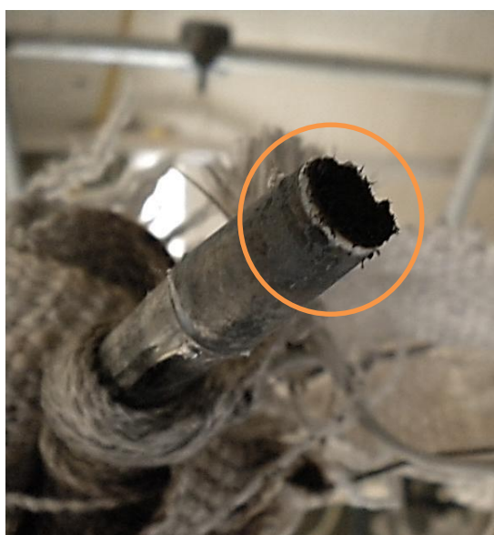
Figure 62: Char in the end of the glass transition pipe
