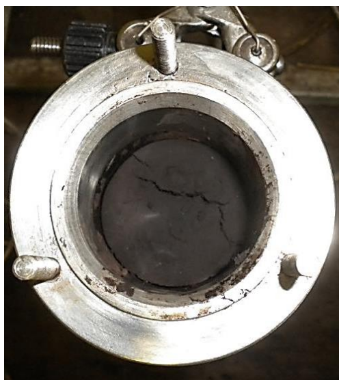
Figure 127: AHR acts as a filter cake for methanol
