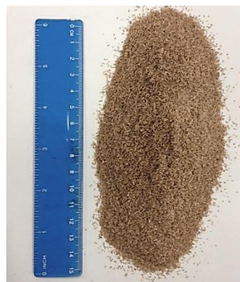
Figure 12: AHR from ground beech: 20 wt.% H 2 SO 4 , 4 hours, 75°C
