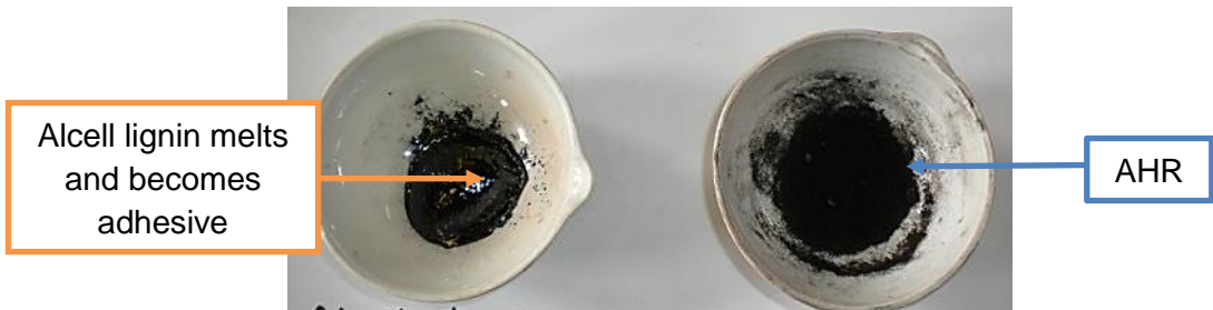
Figure 34: Alcell lignin and AHR after melt test at 400°C
