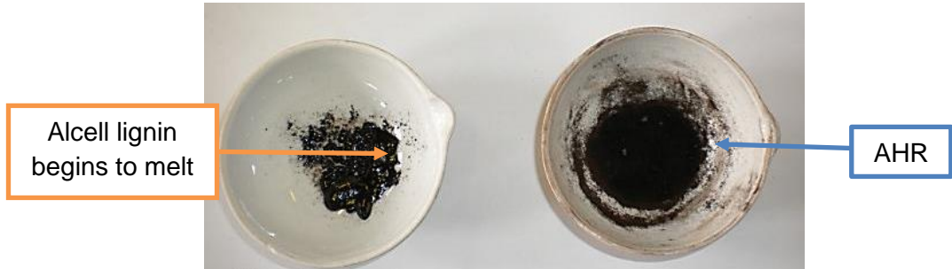
Figure 33: Alcell lignin and AHR after melt test at 300°C
