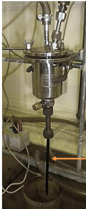
Figure 131: Thread-like feeding which could not be controlled and feeding too fast
