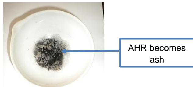
Figure 36: AHR after melt test at 600°C
