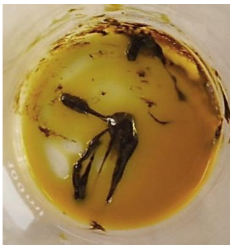
Figure 152: Phase separation when water is added to bio-oil at a 1:1 mass ratio
