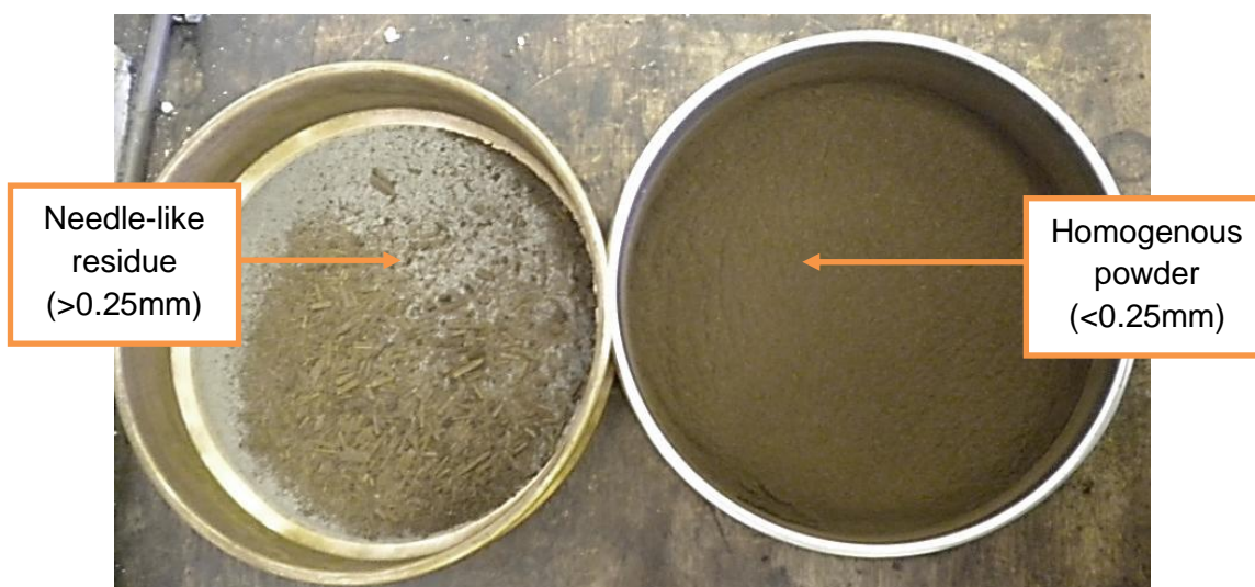
Figure 125: Needle-like AHR on the left and homogenous powder AHR on the right
