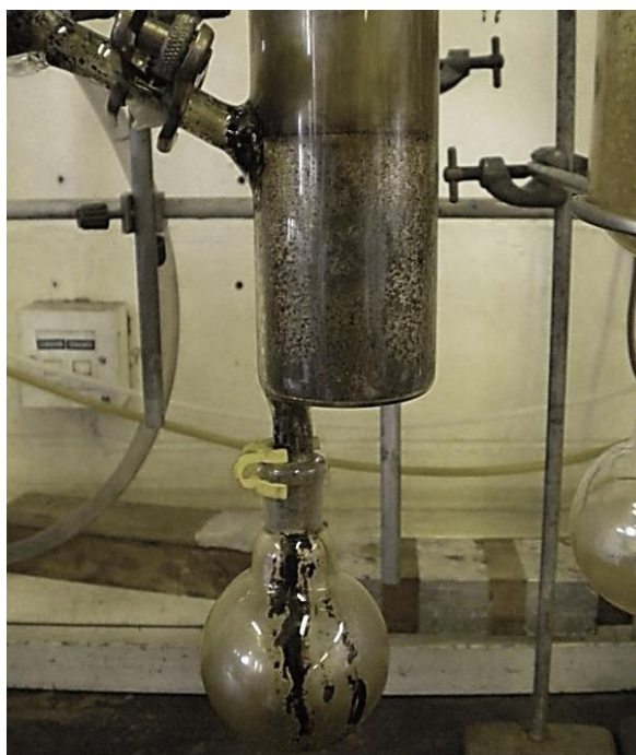
Figure 94: AHR blown out of reactor into the ESP
