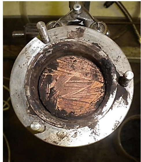
Figure 130: Rubber bung to act as a press on the paste and avoid nitrogen leaving the feeder
