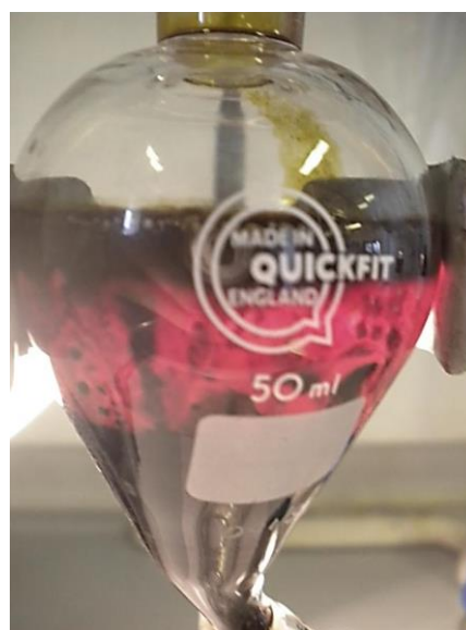
Figure 63: Phase separation in the main oil collection pot
