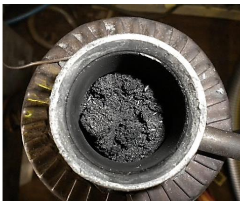
Figure 67: Example of char retained in the reactor
