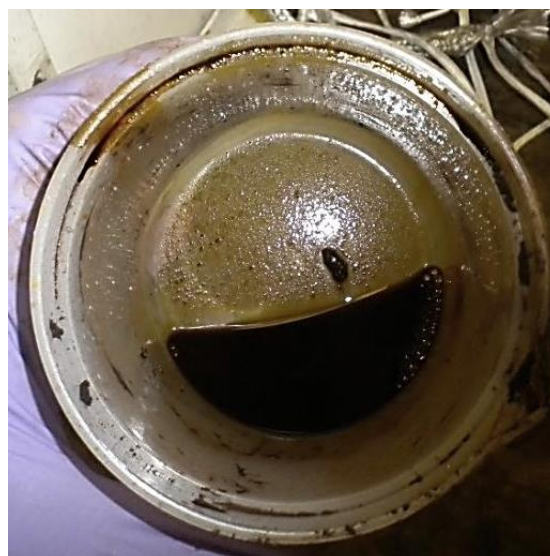
Figure 128: Methanol filtrate is forced through the solid AHR
