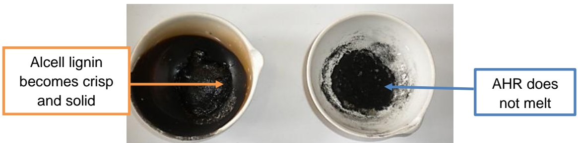
Figure 35: Alcell lignin and AHR after melt test at 500°C
