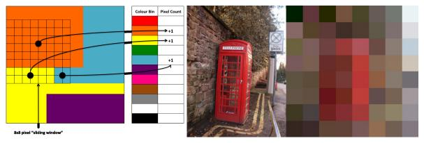
(a) The `sliding window' approach of the MPEG-7 (b) An image partitioned into  $64(8 \times 8)$  blocks represented in the MPEG-Colour Structure Descriptor. 7 Colour Layout Descriptor.
