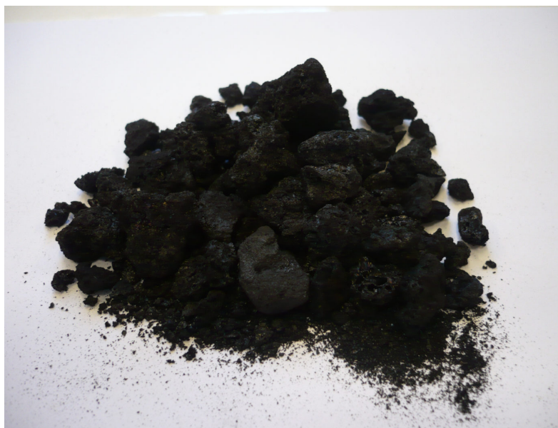
Fig. 6.4 Bio-char from intermediate pyrolysis of Chlorella vulgaris at 500°C
