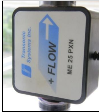
Figure 3-51: Flow sensor used to measure aortic flowrate at ascending aorta
