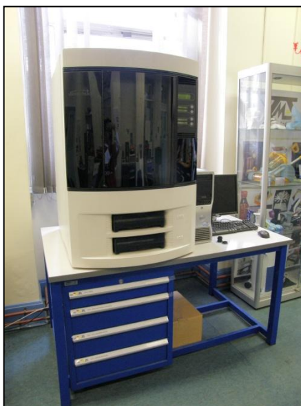
Figure D-142: A rapid prototyping machine (Dimension Elite by Stratasys Inc.) using Fused Deposition Modeling (FDM®) technology.
