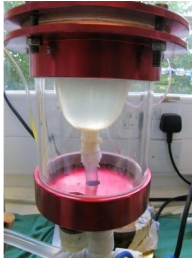
Figure 3-48: Left ventricular chamber with left ventricular silicone sack inside it. Notice the connection to PVC tube from the apex of the silicone sack.
