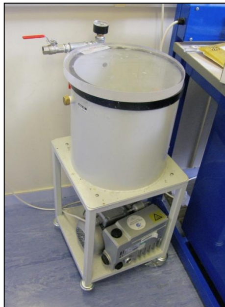
Figure A-136: Degassing chamber capable of vacuum pressure up to -1 bar or -30 mmHg
