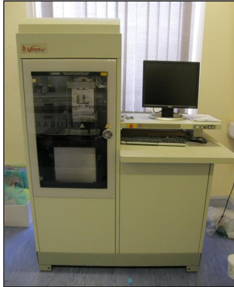
Figure D-143: A rapid prototyping machine (VIPER si2™ SLA® System) to manufacture transparent housing body for balloon pump prototype.
