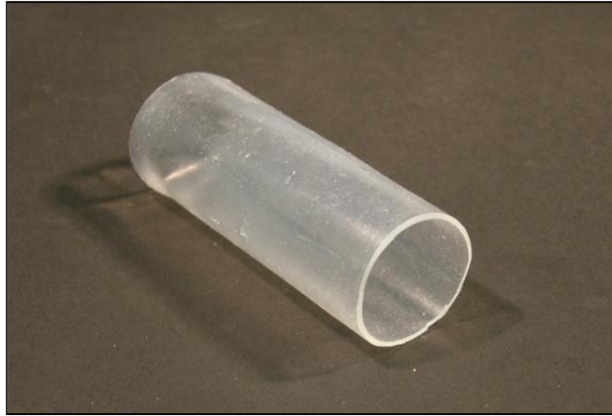
Figure A-140: A cylindrical silicone membrane used in the in vitro prototype balloon pump
