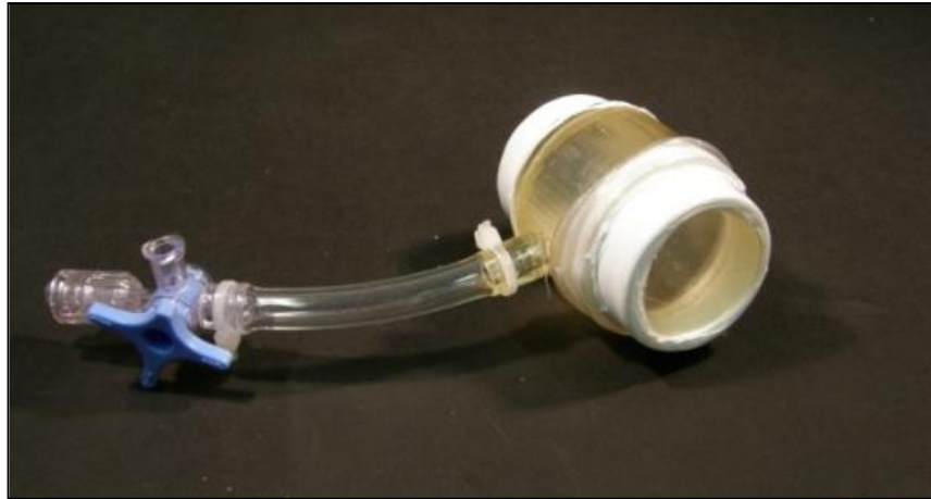
Figure 3-45: Compliant body balloon pump made using a UV-curable photopolymer resin.
