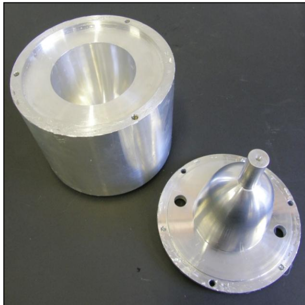
Figure A-141: Mould for the LV silicone sack
