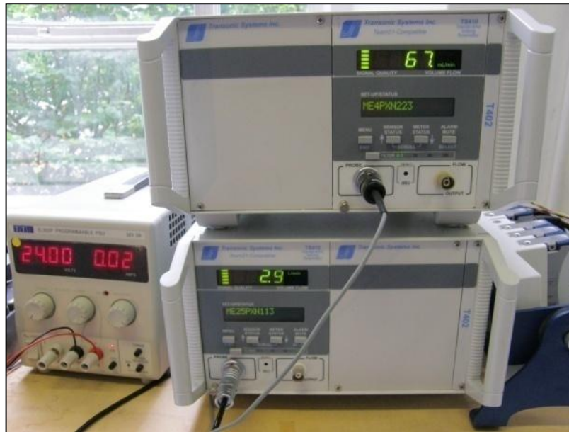
Figure 3-56: TS410 Flowmeter for fluid volumetric measurement. The above flowmeter is for the LCA circulation while the one at the bottom is for the peripheral circulation. The LCD displayed mean flowrate value.
