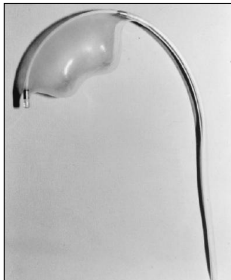
Figure 2-33 : The ascending aortic balloon pump has an oval shape to increase aortic diastolic pressure by occluding the ascending aorta during diastole. (With permission from Elsevier) (B. P. Meyns et al. 2000)
