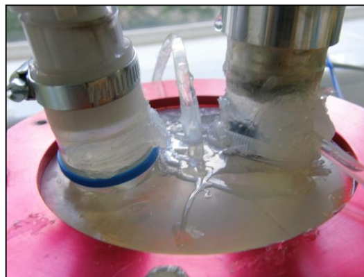
Figure 3-49: LV silicone sack top part that houses heart valves. Notice a tube is inserted at the middle of the top part to measure LV pressure.
