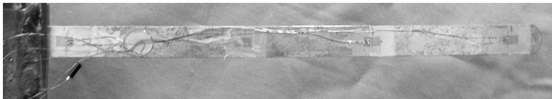
Figure 8: Steel strip with strain gauges
