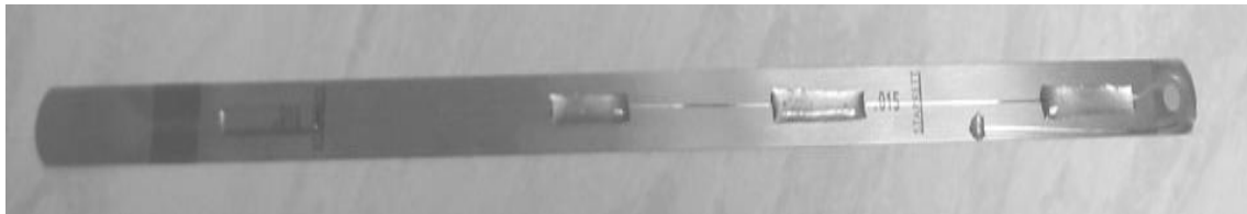
Figure 7: Steel strip with FBG sensors.
