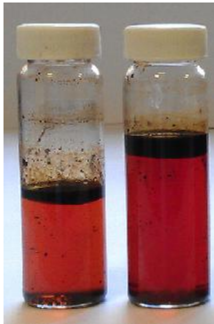
Figure 15: Bio-oil samples recieved different heating rates (left) 25°C/min (right) 100°C/min
