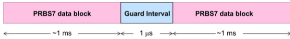
Fig. 5. (Color online) The data frame of the burst switched network consists of a repeating 2^7 - 1 pseudo-random bit sequence (PRBS) of 1 ms duration and a single modified 2^{19} - 1 PRBS of 1 \mu s duration serving as a guard interval.
