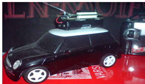
Figure 5. One of the radio controlled cars with the attached mica2 sensor that was used for the In-Motes EYE trial.
