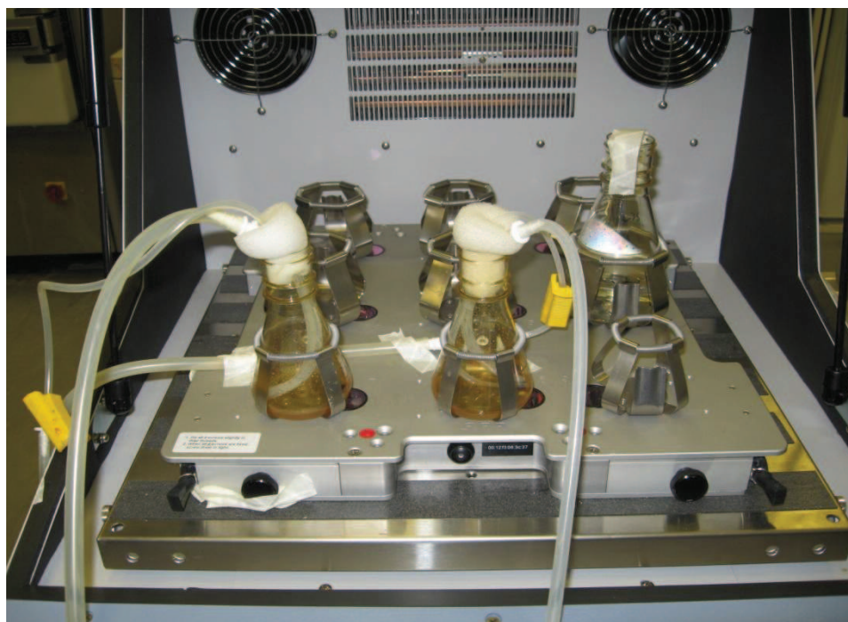
Figure 4.13.: SFR set up for k_La measurements
