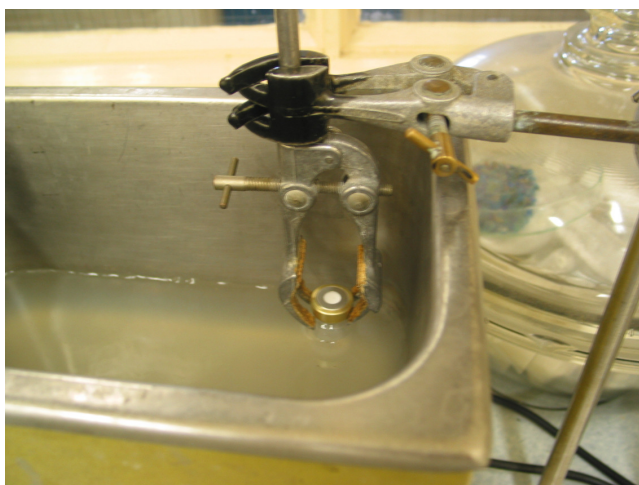
Figure 2.16 Preparation of bubble liposomes. Bubble liposomes were produced by placing SUV liposomes in vials, supercharging with perfluoropropane gas and then placing the vial in a bath sonicator.
