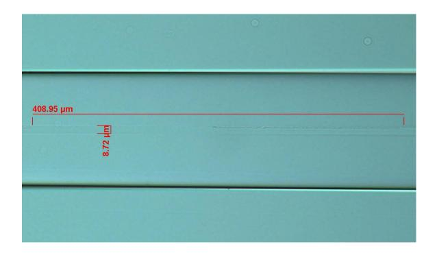
Figure 4-9 showing the femtosecond induced LPG period 400 $\mu$ m showing the measured period to be approximately 408 $\mu$ m
