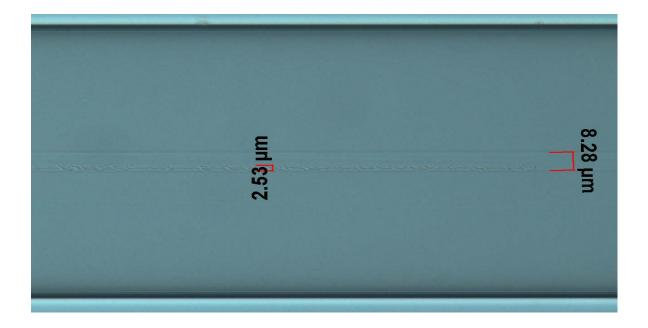
Figure 4-8 showing the femtosecond induced LPG period 400 $\mu$ m showing the RI change to be located on the edge of the core and being approximately 2.5 $\mu$ m wide.
