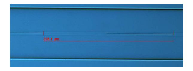
Figure 4-3 showing the femtosecond induced LPG measured period approximately 328µm
