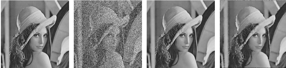
Figure 7: The original image. Noisy image (noise density 50%). Image denoised with linear interpolation and median filter.
