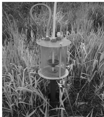
Fig. 4 – Experimental set-up (left) for in-situ determination of the hydraulic conductivity of highly porous media (not to scale) and the apparatus installed at a HSSF TW in the UK (right). Reservoir stands approx. 1 m off the ground. Reproduced from Knowles and Davies (2009).
