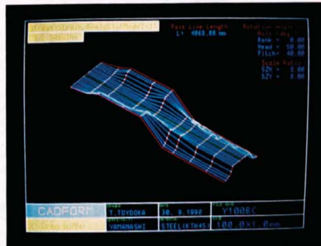
(c) 3-D variation of longitudinal stress \sigma_z
