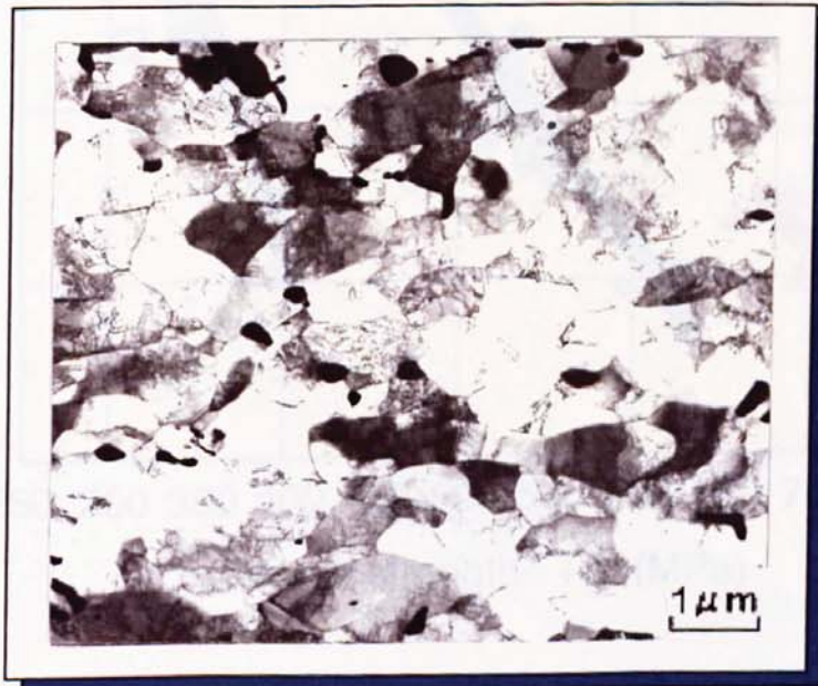
(c) Scanning electron microstructure of HISTORY steel tube
