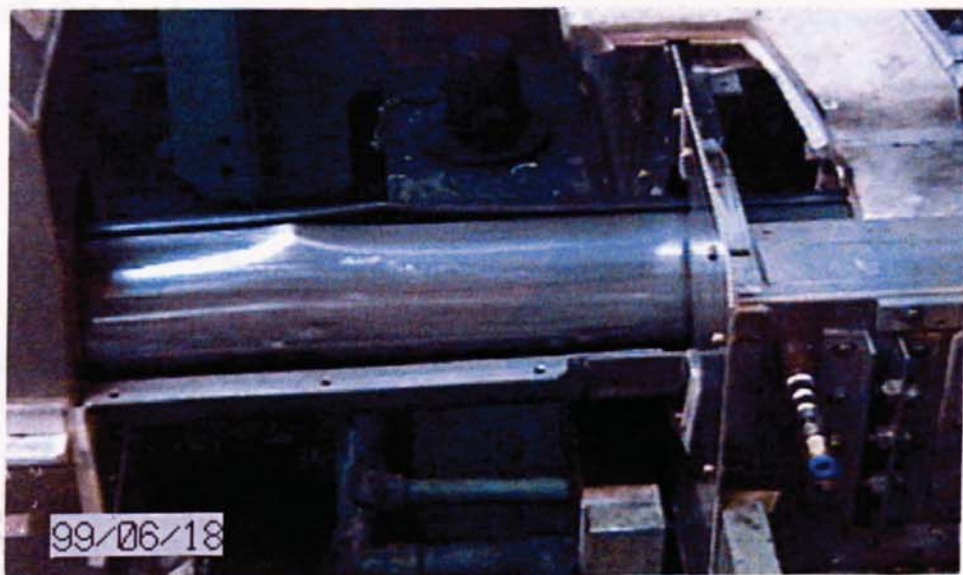
Photo.6 Appearance of edge buckling in actual production of thin walled pipe with D = 146.0\text{mm} , t = 2.0\text{mm} and \sigma_Y = 730\text{MPa} .
