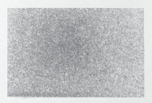
Figure 29 Metallographic microstructure of water quenched and tempered steel magnification X100.
