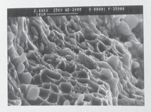
Figure 55 SEM details of fracture surface for tensile test specimen with a defective weld magnification X 2.6 K
