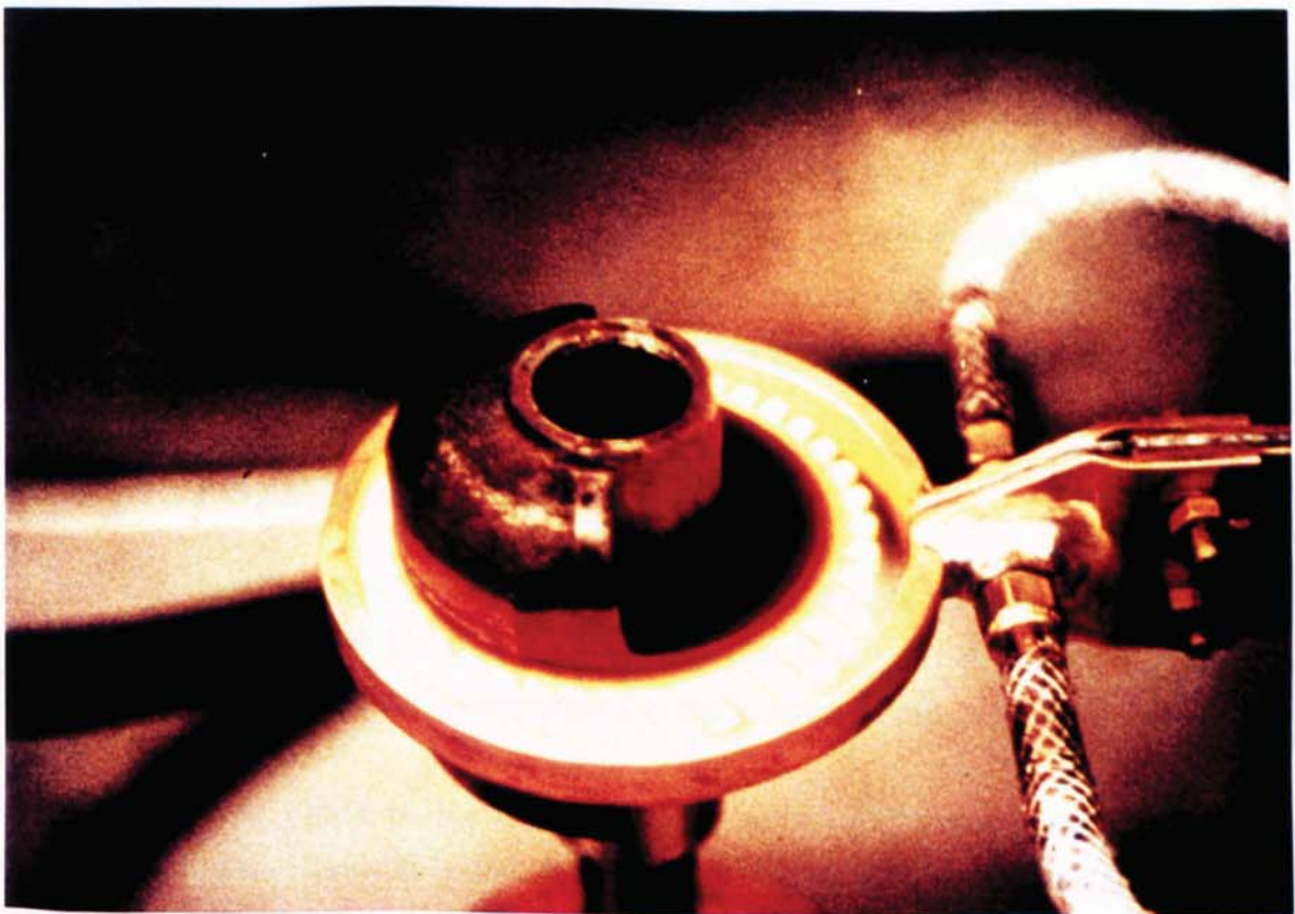
Figure 1.3 Induction Hardening of Gear Wheel Teeth
