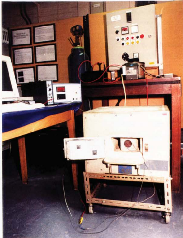
Figure 4.8 Photograph of Furnace and Strain Gauge Equipment.
