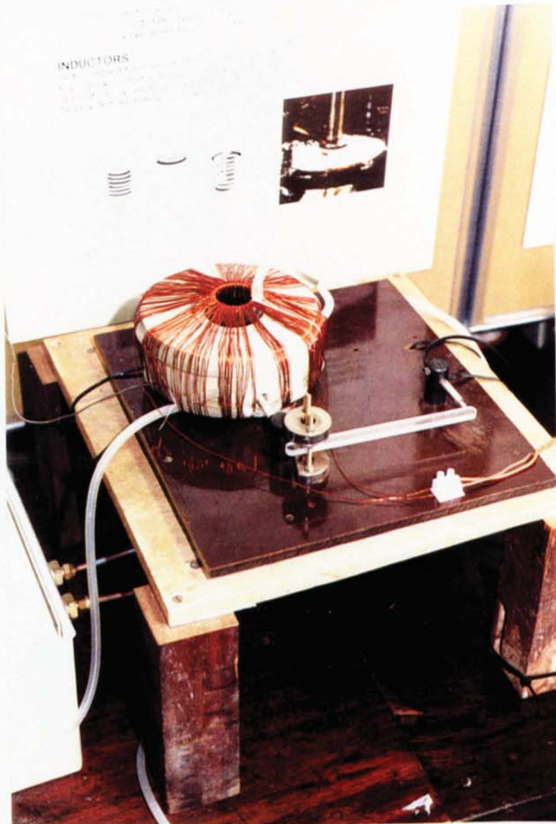
Figure 4.2 Photograph of Apparatus Used to Measure Magnetostriction
