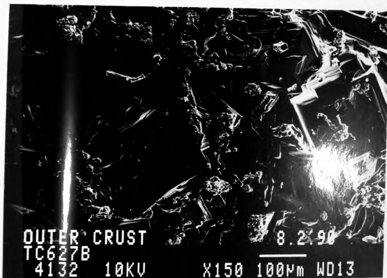
Plate 6.5 Inner and Outer Crust Surface of a 40% Weight Sodium Chloride Drop (63.5°C, 1m/s).
