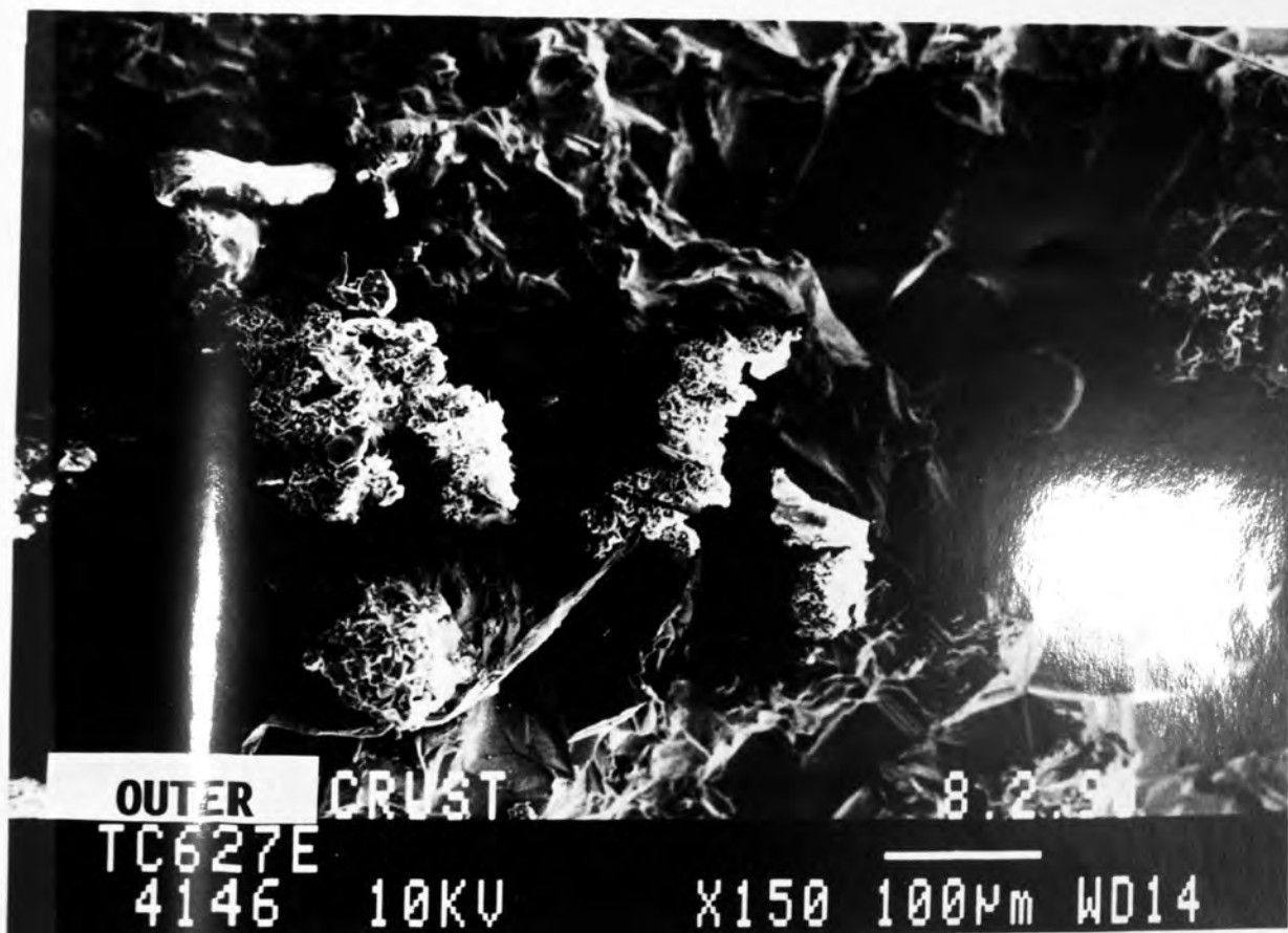
Plate 6.4 Inner and Outer Crust Surface of a 40% Weight Sodium Chloride Drop (54°C, 1m/s).
