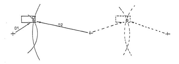
NOTE: TWO RECIEVERS REQUIRED TO DEFINE UNIQUE VEHICLE POSITION COMPUTED DISTANCE D1. D2 PROVIDE THE VEHICLE WITH REQUIRED INFORMATION FOR POSITION IDENTIFIFCATION
