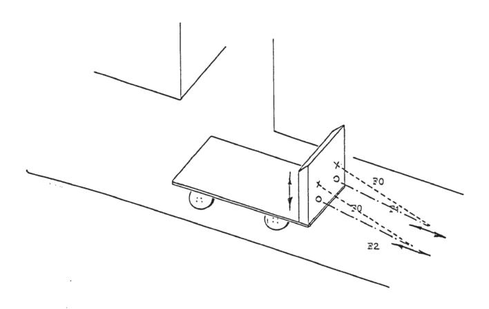
VEHICLE VELOCITY = FUNCTION (FO - F1)+(FO - F2) DISTANCE =  $\int V dt$ TURNING MOTION = FUNCTION (F1 - F2)
