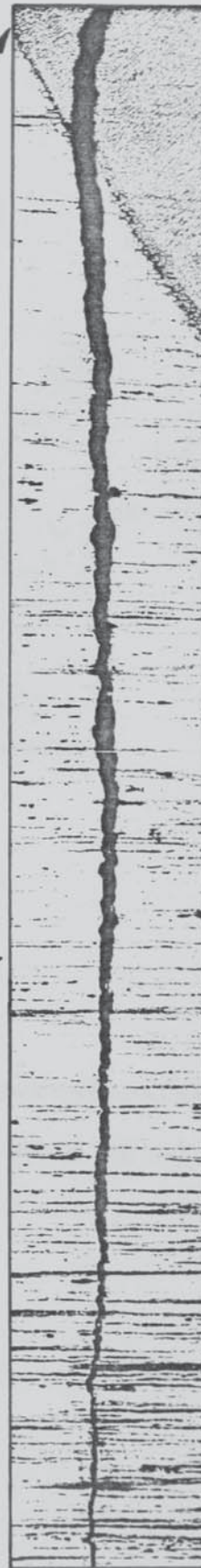
Figure 6.12 : Fatigue crack profile showing crack facets
