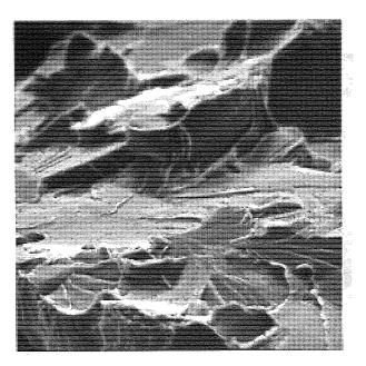
Plate 47 Steel A(1277). Fracture surface next to the fatigue crack tip. SEM (x1.45K)
