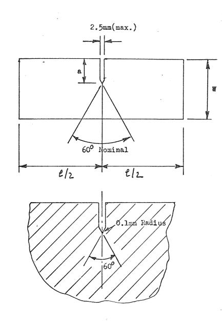
Fig. 6.3 Three Point Bend Specimen.
