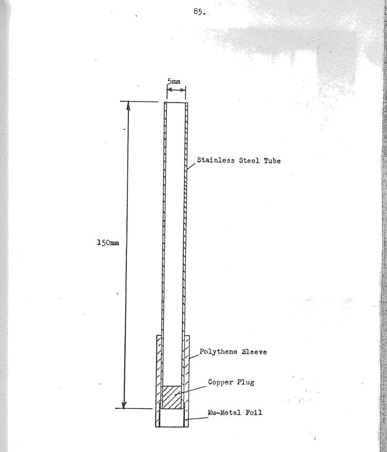
Fig. 6.7 The Cathode used in the Electropolishing Method.
