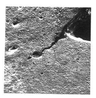
Plate 54 Steel F. Crack path. SEM (x260)
