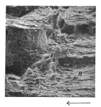
Direction of crack propagation Plate 38 Steel L. Fracture surface at the fatigue crack tip. A-fatigue area, B-small dimples and C-tearing. SEM(x650)
