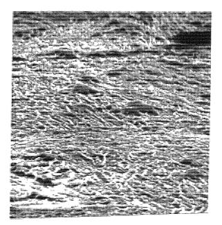
Plate 19 Microstructure of Material C at the centre of the block. Electro-etching.Scanning Electron Micrograph (x2.4K)
