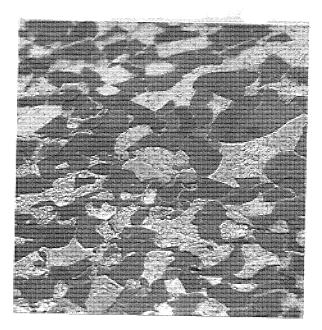
Plate 40 Steel A. Microstructure, conventional etching (x650)
