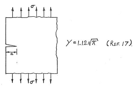
b) Surface crack in a semi-infinite plate.
