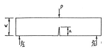
$\gamma(^{\circ}_{W}) = 1.93 - 3.07(^{\circ}_{W}) + 14.53(^{\circ}_{W})^{2} - 25.11(^{\circ}_{W})^{3} + 25.8(^{\circ}_{W})^{4}$ (REF. 18) c) Surface crack in a three-point bend specimen.
