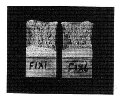
Plate 50 Fracture surfaces of 20mm thick specimen from Steel F.
