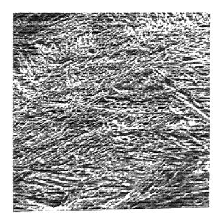
Plate 21 Microstructure of Material C at the corner of the block. Electro-etching.Scanning Electron Micrograph (x2.4K)
