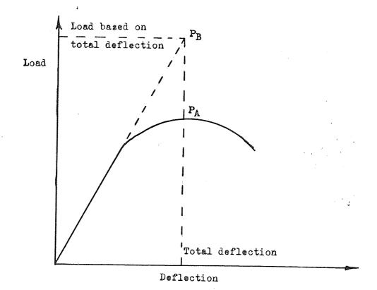
Fig. 3.3 Method used to determine load used in scaling method. (Ref. 24)
