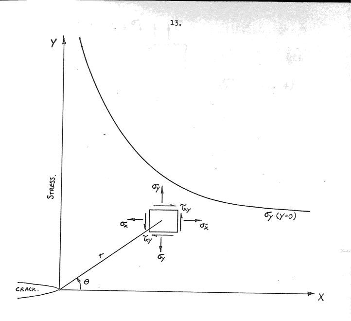
Fig. 2.2 Schematic illustration of the elastic stress distribution near the tip of a crack.
