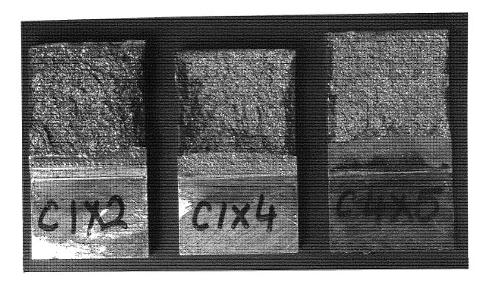
Plate 17 Fracture surfaces from 25mm thick specimens of Steel C.
