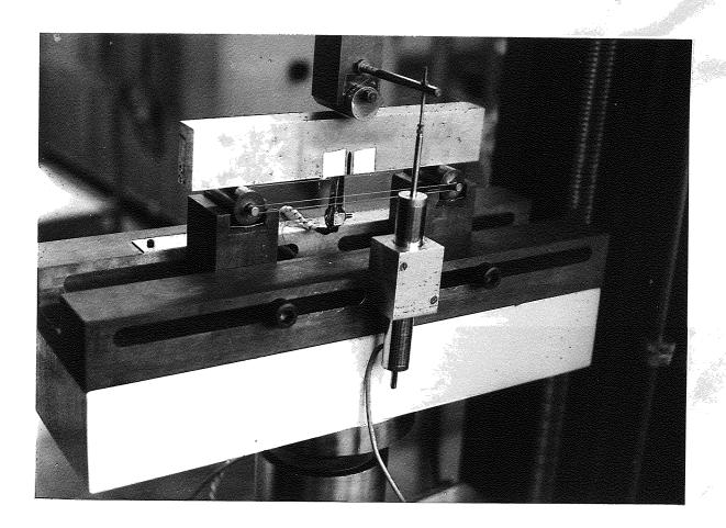
Plate 3 Test Rig for Three-Point Bend Tests showing the Load Point Displacement Transducer.
