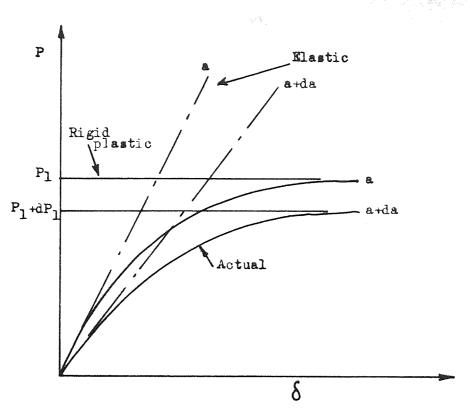
(a) Typical load-displacement (P v's  $\delta$ ) records.
