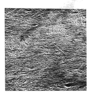
Plate 20 Microstructure of Material C at the corner of the block. Electro-etching.Scanning Electron Micrograph (xl.2K)
