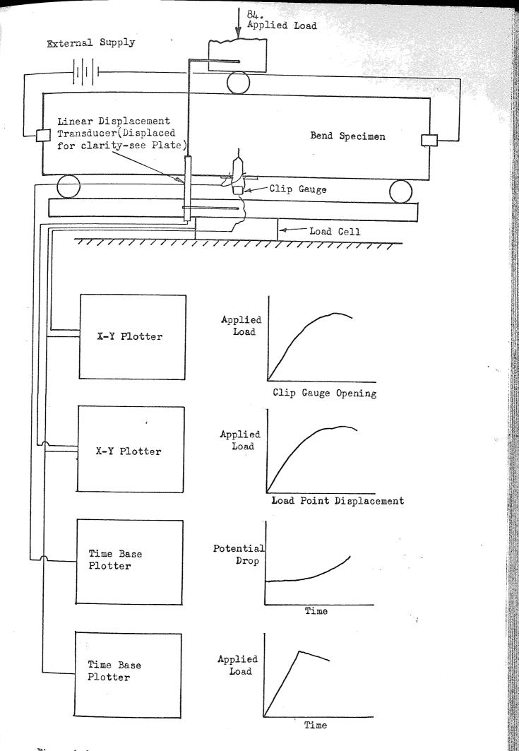
Fig. 6.6 Schematic Arrangement of Recording Equipment on Fully Instrumented Fracture Toughness Test.
