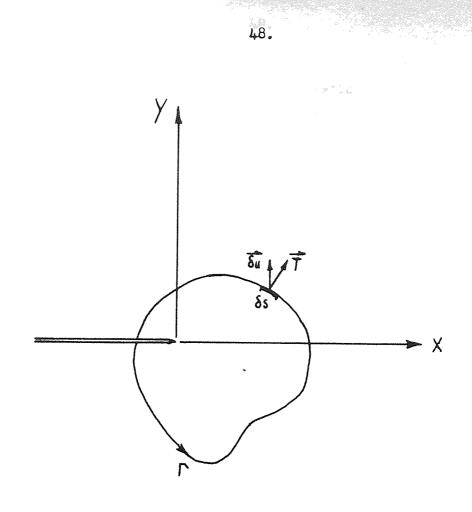
Fig. 4.4 Crack tip coordinate system and arbitrary line integral contour.(Ref. 49)
