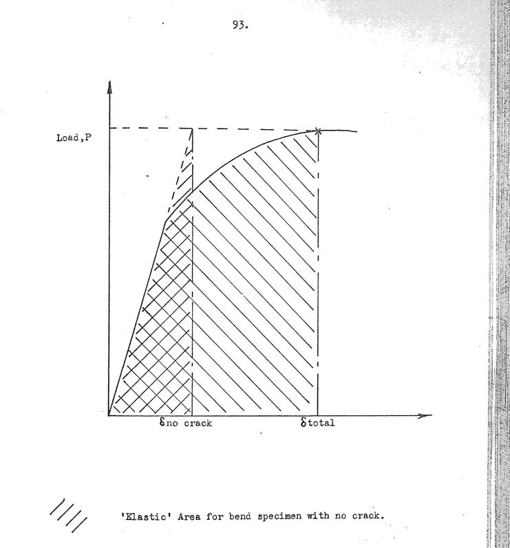
'Elastic' Area for bend specimen with no crack.
