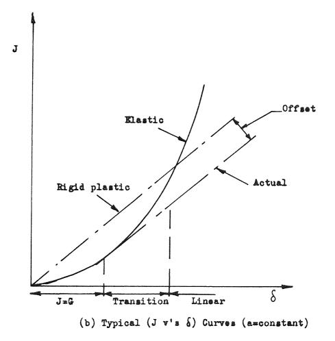
Fig. 4.5 Idealised versus actual behaviour for load-displacement and J-displacement.(Ref.56)
