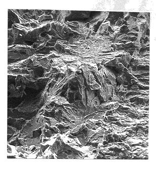
Direction of crack propagation Plate 8 Material M - Fracture surface at the fatigue crack tip showing cleavage fracture.Scanning Electron Fractograph (x280)
