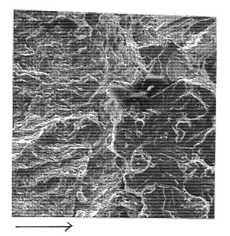
Plate 25 Material C. Fracture surface at the fatigue crack tip showing mixed fracture mechanisms of cleavage and microvoid coalescence.Scanning Electron Fractograph(x600)
