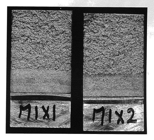
Plate 4 Fracture surfaces from 25mm thick specimens of Steel M.
