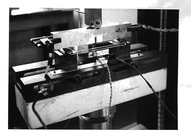
Plate 2 Three-Point Bend Rig showing Potential Drop Apparatus.
