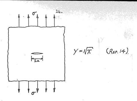
a) Isolated crack in an infinite plate.
