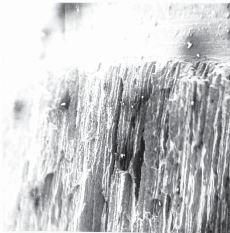
Figure 81 Final Fracture Appearance of Parent Plate Material S.E.M. x 21
