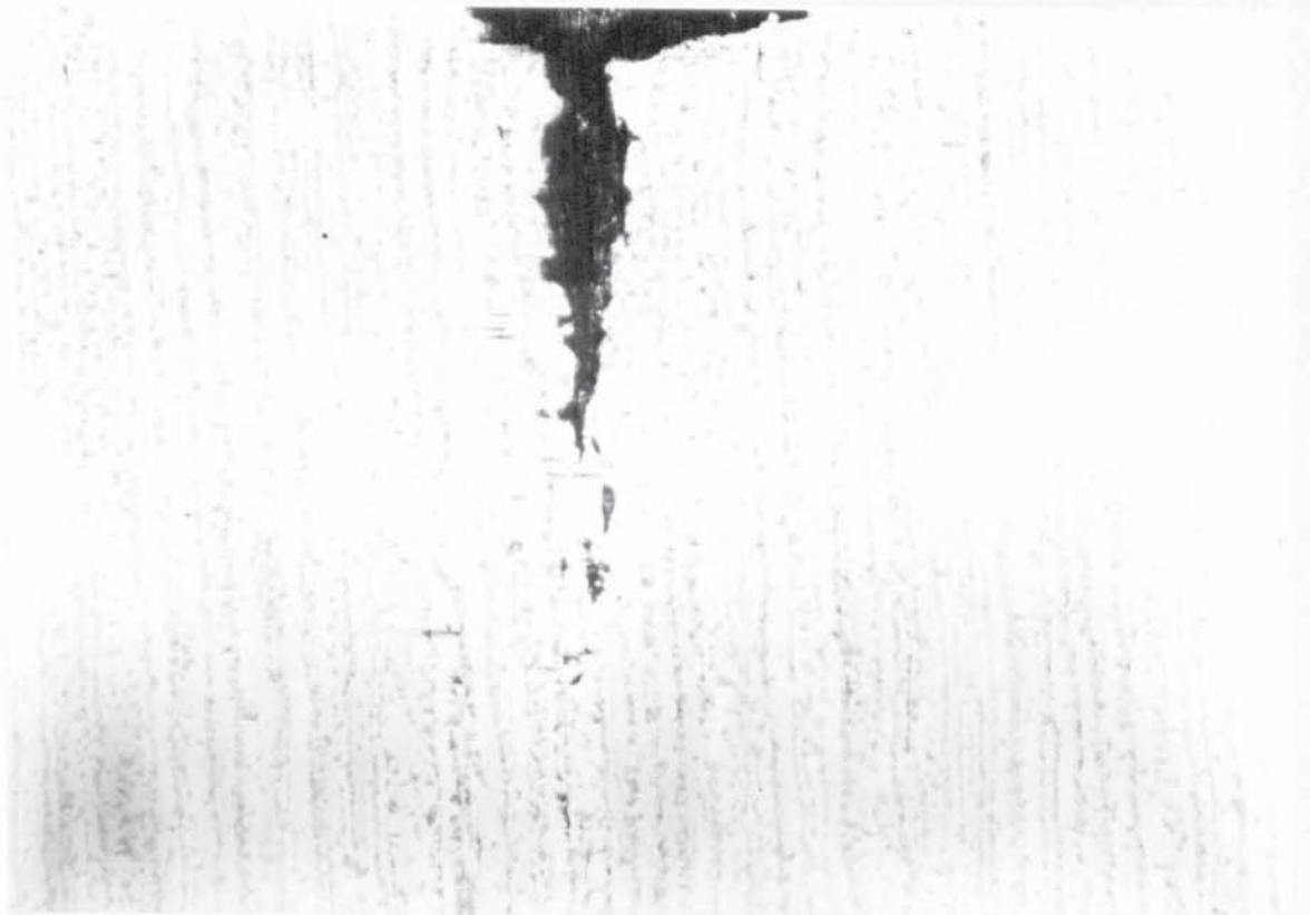
Figure 79 Growing Crack x 50
