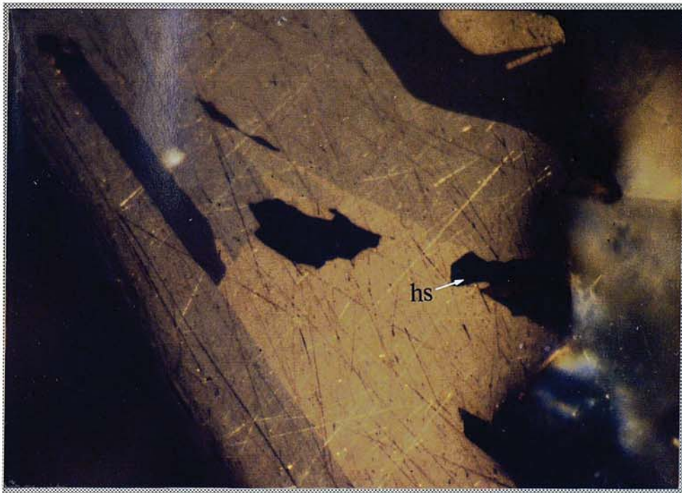
Plate 4.23b. Crossed polars view of figure 4.23a with the hessite (hs) exhibiting blue-red anisotropy colours (field of view 225 \mu m, oil, X-polars).
