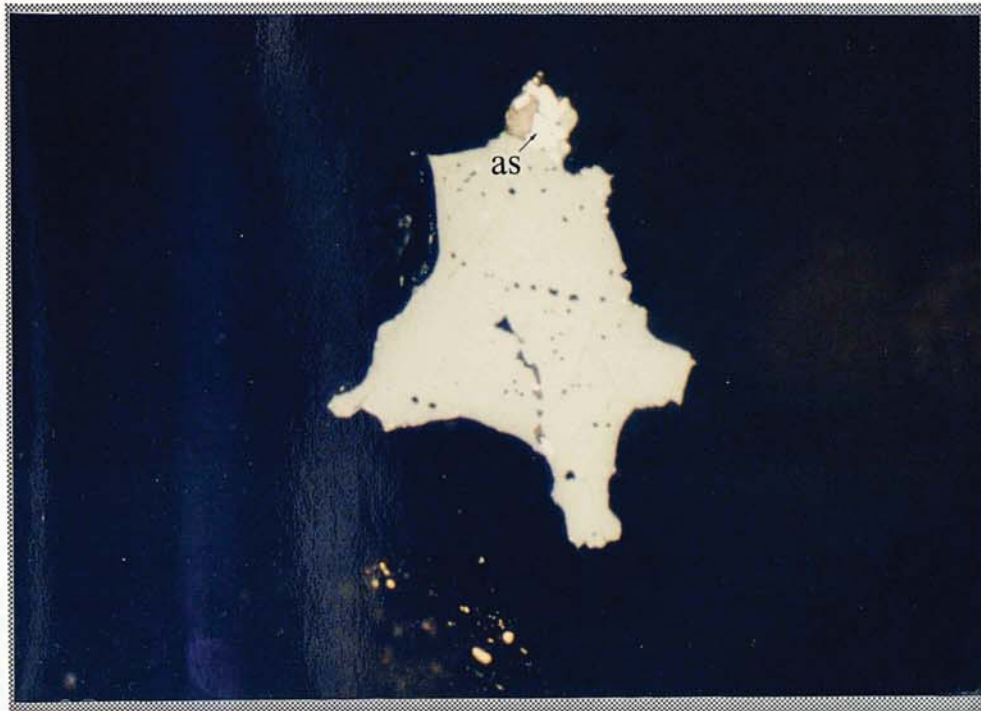
Plate 4.38. Tetrahedrite in a vug in quartz. The small inclusions in the tetrahedrite are arsenopyrite (as) (field of view 225 \mu m, oil, PPL, sample number: K2).
