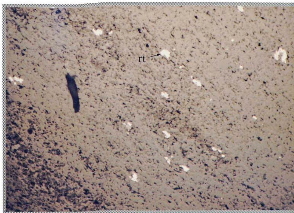
Plate 4.4. Small rutile grains (rt) in shale inclusion (field of view 1125 \mu m, air, PPL, sample number: SB 128 B).
