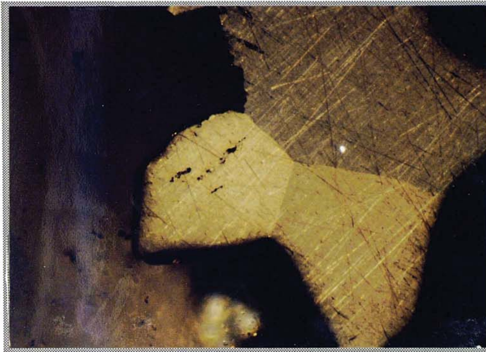
Plate 4.11. Triple point grain boundaries in tellurbismuth (field of view 560 \mu m, oil, X-polars, sample number: JN 5 ).
