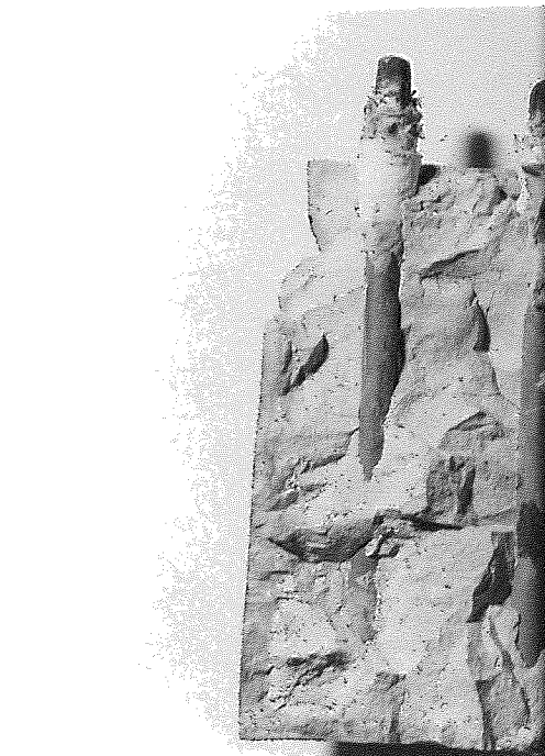
Figure 8.10 Photograph showing corrosion of steel embedded in polymer impregnated OPC/BFS paste of 0.6 water/cement ratio cured under cc(1) kept at 50%RH and 40°C.
