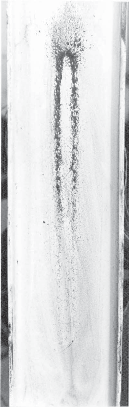
Plate 9 Unstiffened secondary beam-to-column connection showing the yield lines on the column web at ultimate load.
