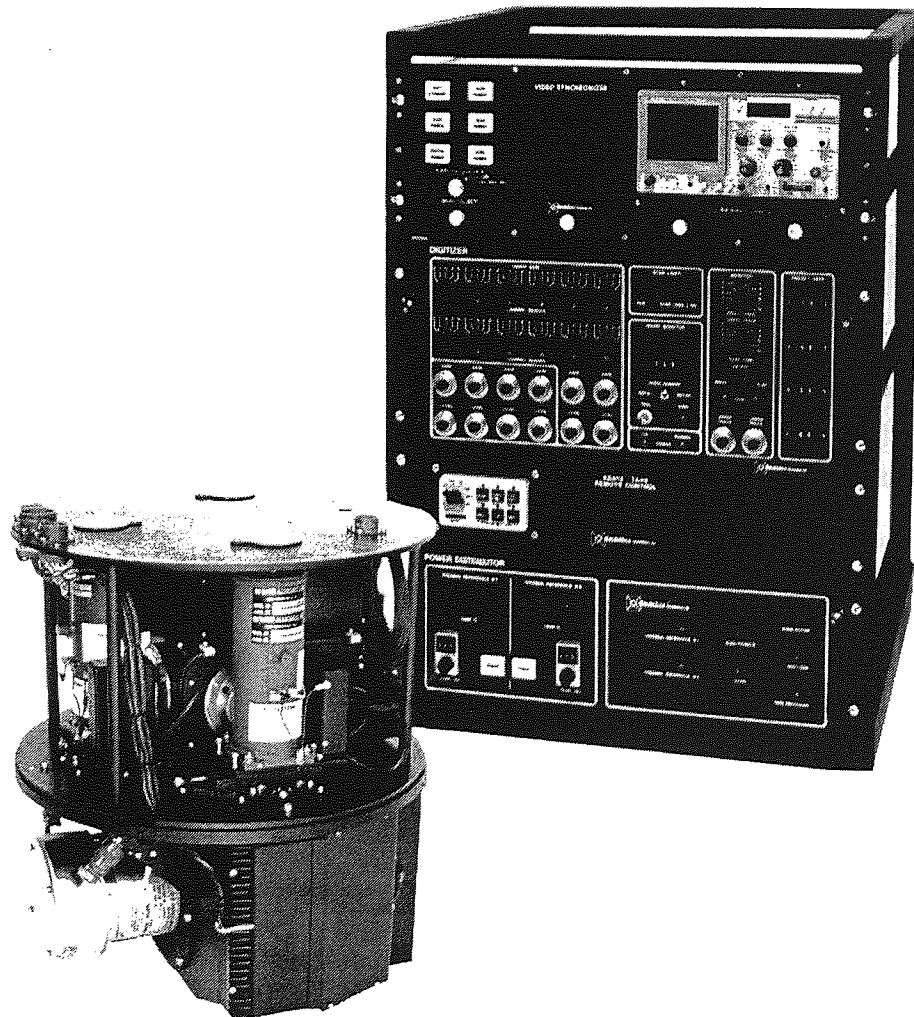
Figure 4.12. The Airborne Thematic Mapper with the scanning head (left) and the control unit (right).
