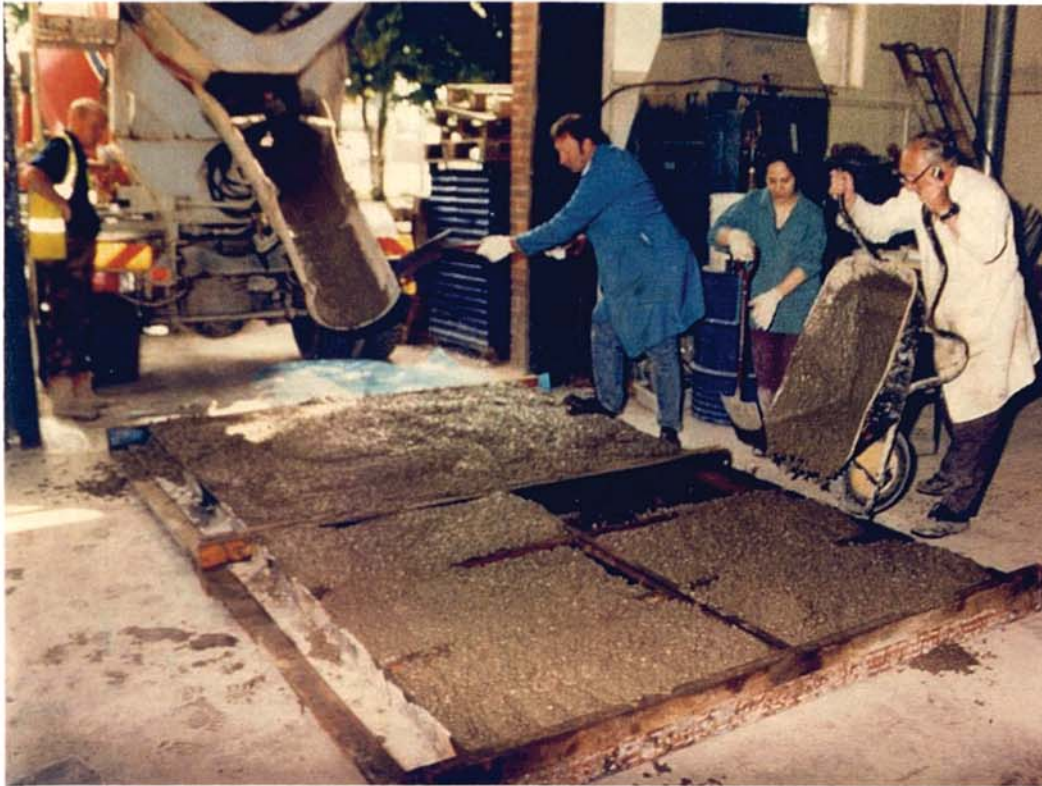
Plate 9.5 Fabrication of ready mix concrete specimens
