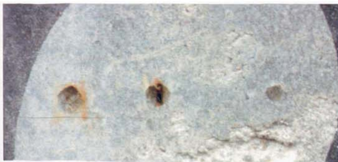
Plate 8.4 Example of ball craters on a typical concrete sample
