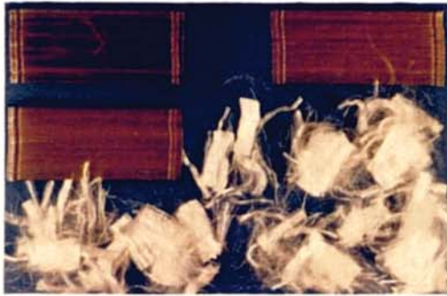
Plate 4.9 Blend of steel and polypropylene fibres
