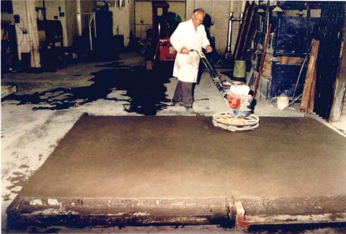
Plate 9.7 Power finishing of ready mix concrete specimens
