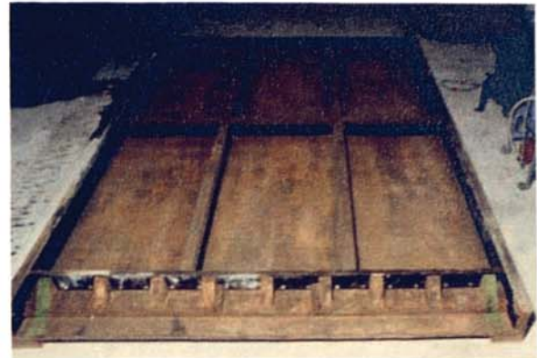
Plate 5.4 Empty mould internally subdivided into six sections
