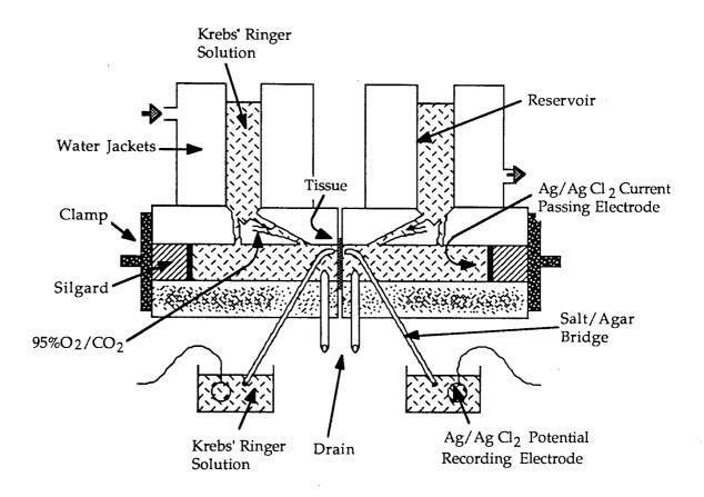
FIGURE 7: A diagrammatic representation of the Ussing chamber used in the present investigation. The equipment comprised of two interlocking perspex half chambers with bathing fluid reservoirs surrounded by water jackets (refer to text for details).
