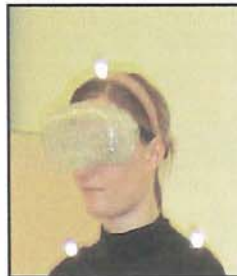
Figure 5:1 Opaque goggles worn to remove visual cues to orientation. Goggles are secured with elastic and are adjustable in size.
