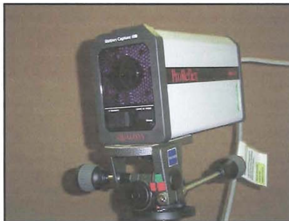
Figure 4:3 Qualisys Systems ProReflex™ Motion Capture MCU 120 camera.
