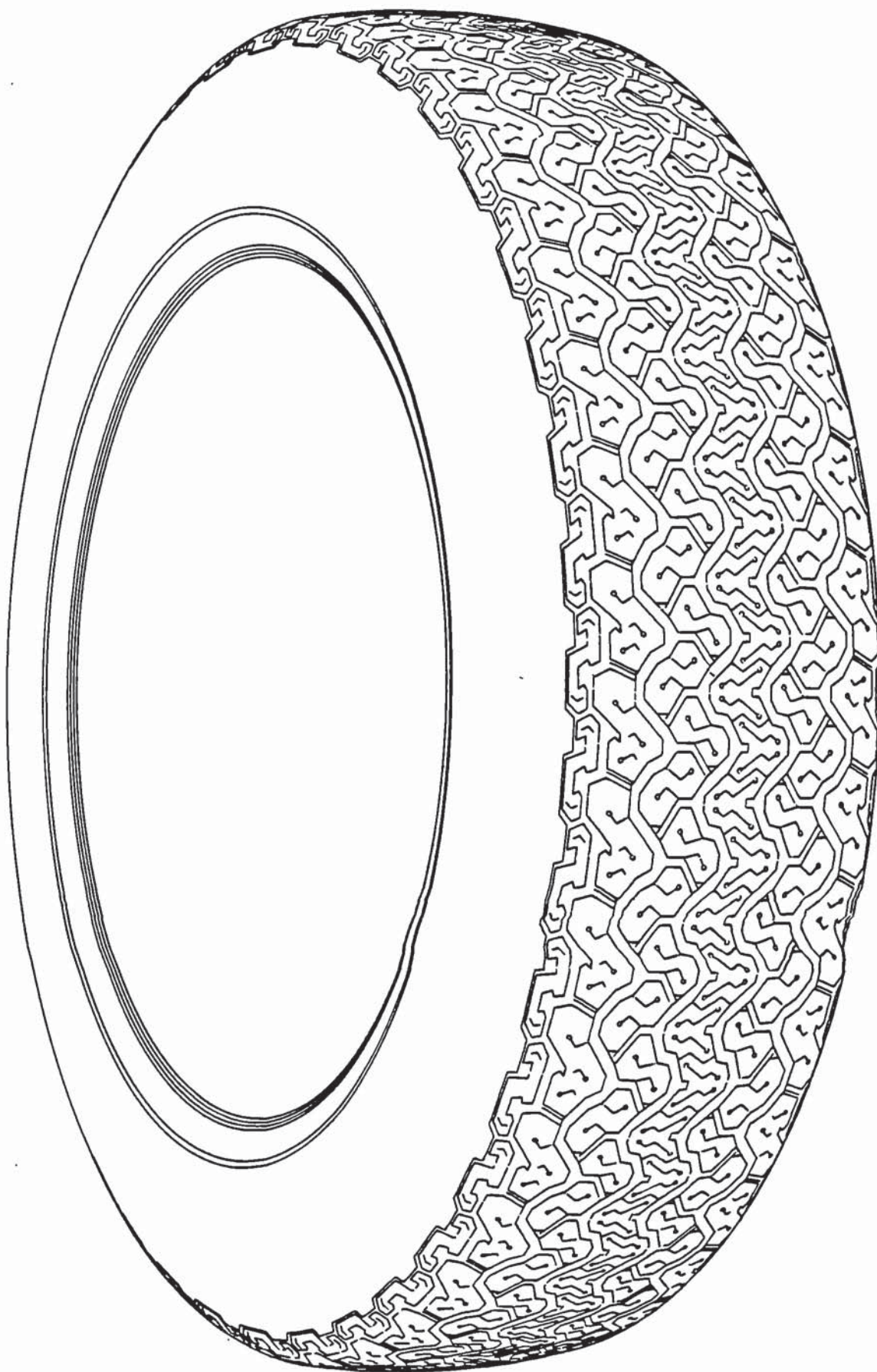
TREAD PATTERN - COMPUTER DRAFTED - 185/70HR13 D1 TYRE Figure 7.3.
