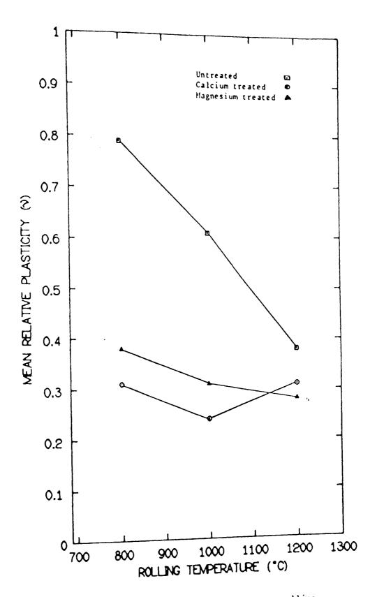
FIGURE 36 Mean relative plasticity versus rolling temperature
