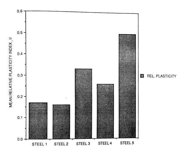
FIGURE 42. MEAN RELATIVE PLASTICITY INDICES FOR STEELS 1-5 (CONTROLLED ROLLED)
