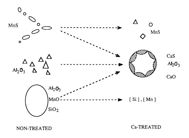
FIGURE 9. Schematic presentation showing modification of inclusions with calcium treatment <sup>78</sup>.
