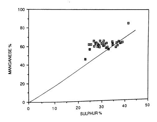
FIGURE 96. MANGANESE VERSUS SULPHUR CONTENT FOR THE INCLUSIONS IN STEEL 5.
