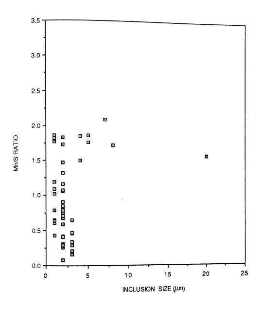
FIGURE 64. Mr/S RATIO VERSUS SIZE FOR THE INCLUSIONS IN STEEL 2.
