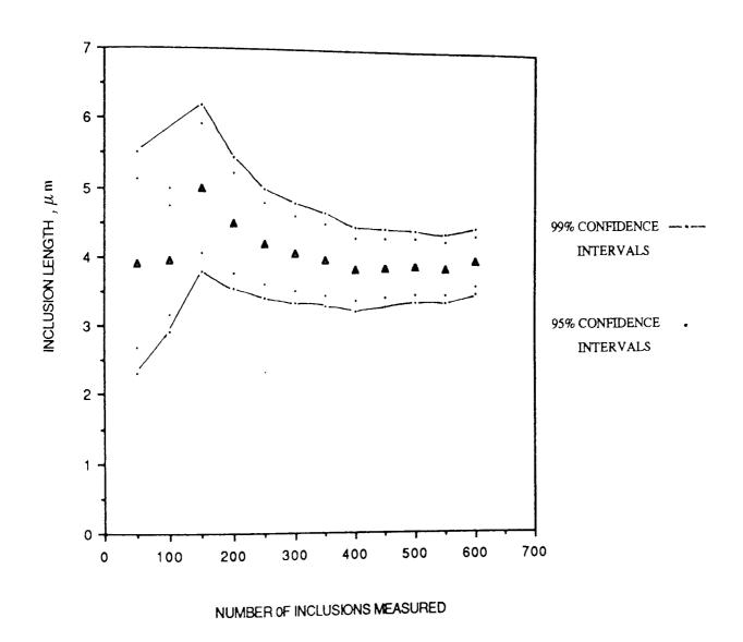
FIGURE 46. MEAN INCLUSION LENGTH VERSUS NUMBER OF INCLUSIONS MEASURED IN STEEL 3.
