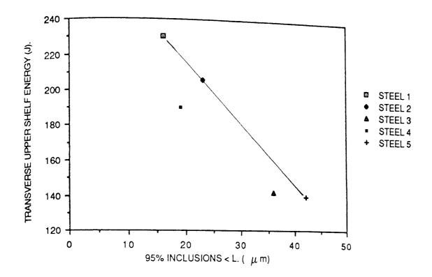
FIGURE 102. TRANSVERSE UPPER SHELF ENERGY VERSUS INCLUSION LENGTH DISTRIBUTION FOR STEELS 1-5 (Thirty Largest Inclusions)
