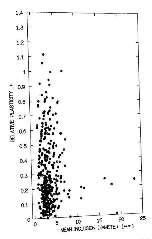
FIGURE 31 RELATIVE PLASTICITY OF THE INCLUSIONS IN THE 0.013% SULPHUR MAGNESIUM TREATED STEEL ROLLED AT 1000°C
