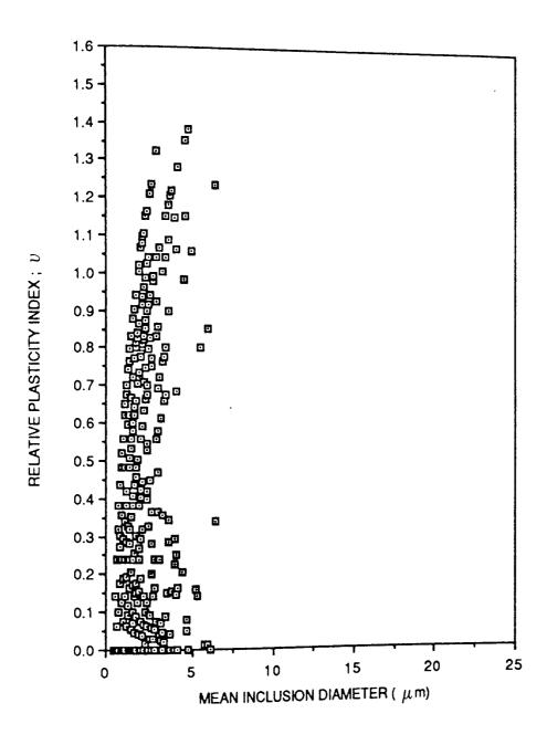
FIGURE 39. RELATIVE PLASTICITY INDEX VERSUS SIZE FOR STEEL 3. (CONTROLLED ROLLED)
