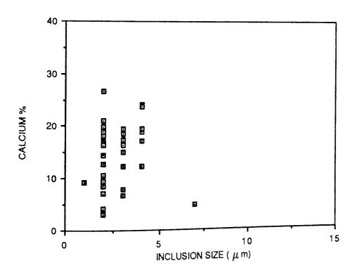
FIGURE 69. INCLUSION SIZE VERSUS CALCIUM CONTENT FOR STEEL 3.
