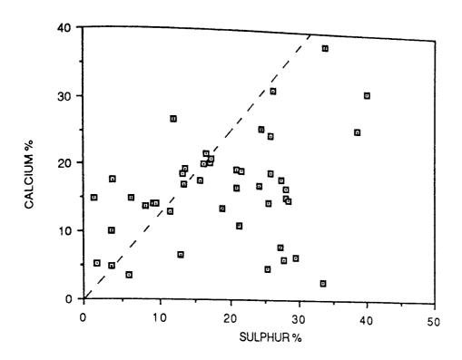
FIGURE 84. CALCIUM VERSUS SULPHUR CONTENT FOR THE INCLUSIONS IN STEEL 2.
