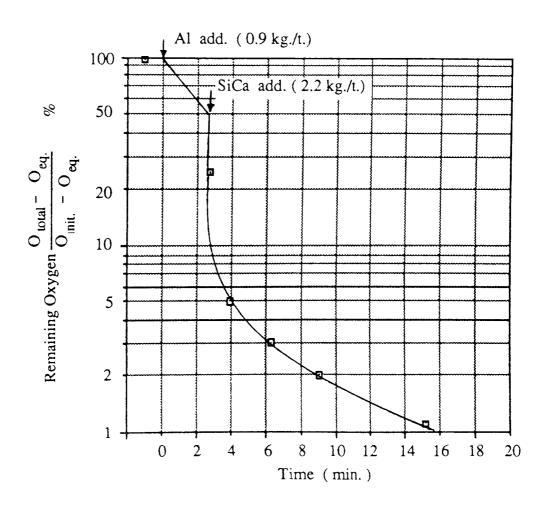
FIGURE 6. Deoxidation by successive additions of aluminium and calcium-silicon alloy<sup>70</sup>
