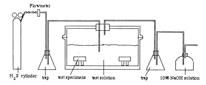
FIGURE 16. Schematic diagram of H.I.C. test assembly.
