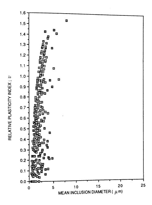
FIGURE 41. RELATIVE PLASTICITY INDEX VERSUS SIZE FOR STEEL 5 (CONTROLLED ROLLED)
