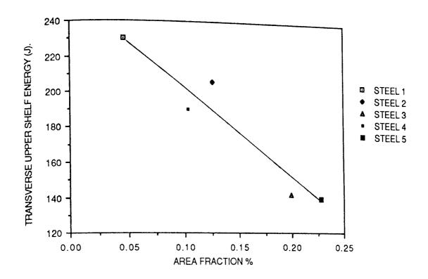
FIGURE 100. TRANSVERSE UPPER SHELF ENERGY VERSUS INCLUSION AREA FRACTION FOR STEELS 1-5.
