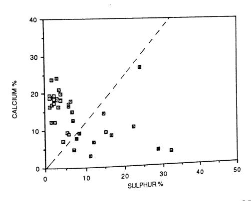
FIGURE 87. CALCIUM VERSUS SULPHUR CONTENT FOR THE INCLUSIONS IN STEEL 3.
