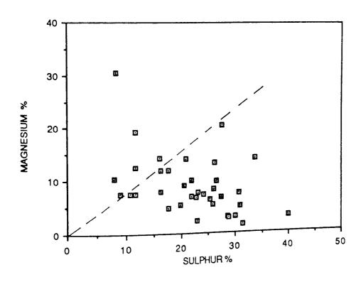
FIGURE 91. MAGNESIUM VERSUS SULPHUR CONTENT FOR THE INCLUSIONS IN STEEL 4.
