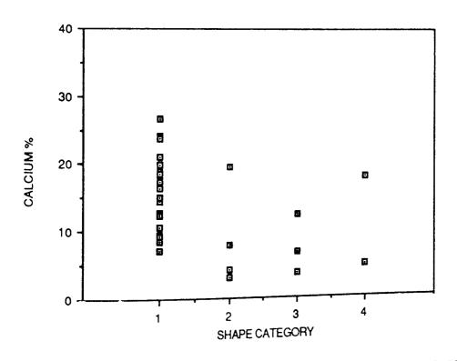
FIGURE 71. INCLUSION SHAPE VERSUS CALCIUM CONTENT FOR STEEL 3.
