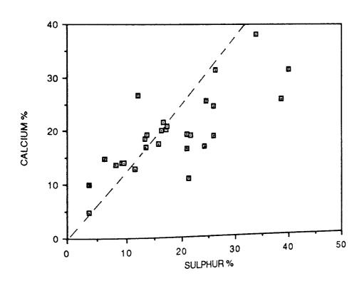
FIGURE 85. CALCIUM VERSUS SULPHUR CONTENT FOR THE INCLUSIONS IN STEEL 2.
