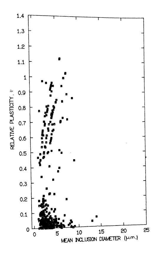
FIGURE 28 RELATIVE PLASTICITY OF THE INCLUSIONS IN THE 0.012% SULPHUR CALCIUM TREATED STEEL ROLLED AT 1000°C
