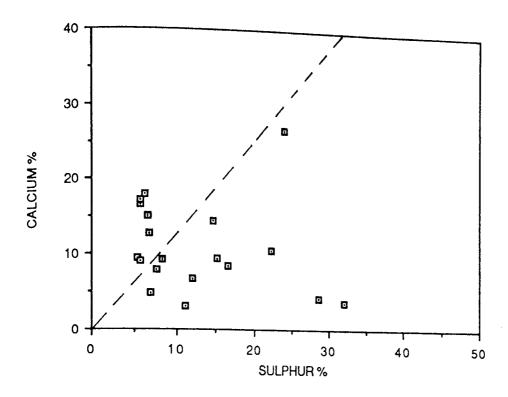
FIGURE 88. CALCIUM VERSUS SULPHUR CONTENT FOR THE INCLUSIONS IN STEEL 3.
