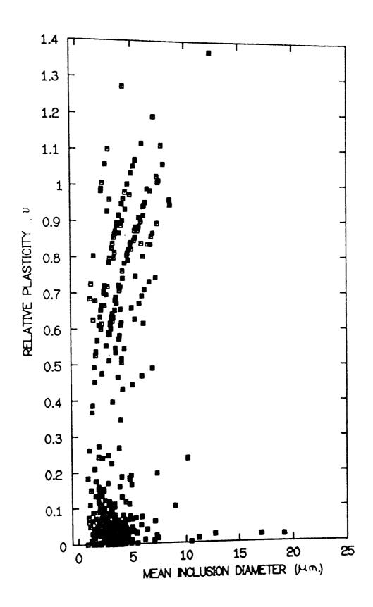
FIGURE 27 RELATIVE PLASTICITY OF THE INCLUSIONS IN THE 0.012% SULPHUR CALCIUM TREATED STEEL ROLLED AT 800°C
