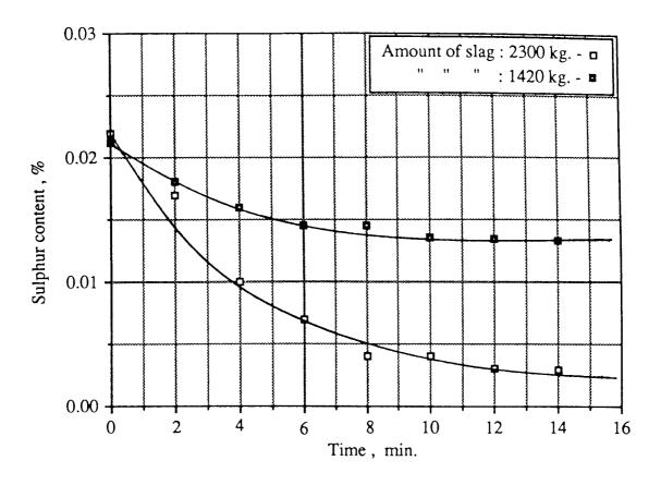
FIGURE 3. Process of desulphurisation on 120-t melts under slag by stirring with argon and the influence of the amount of slag (dolomite ladle)<sup>45</sup>
