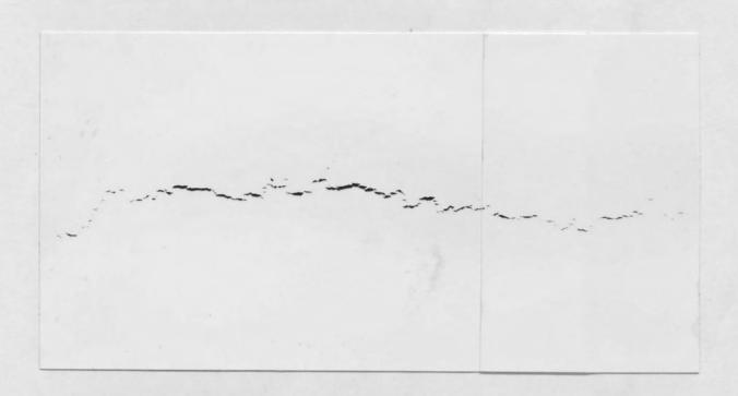
Figure 104. Hydrogen induced 'stepwise' crack found in steel 5.
