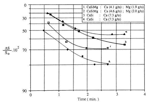
FIGURE 11. Desulphurising by Ca- and Mg- injection as a function of injection time <sup>88</sup>
