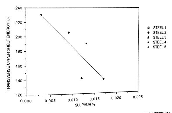
FIGURE 99. TRANSVERSE UPPER SHELF ENERGY VERSUS SULPHUR CONTENT FOR STEELS 1-5.
