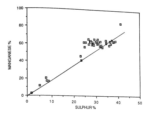
FIGURE 95. MANGANESE VERSUS SULPHUR CONTENT FOR THE INCLUSIONS IN STEEL 5.
