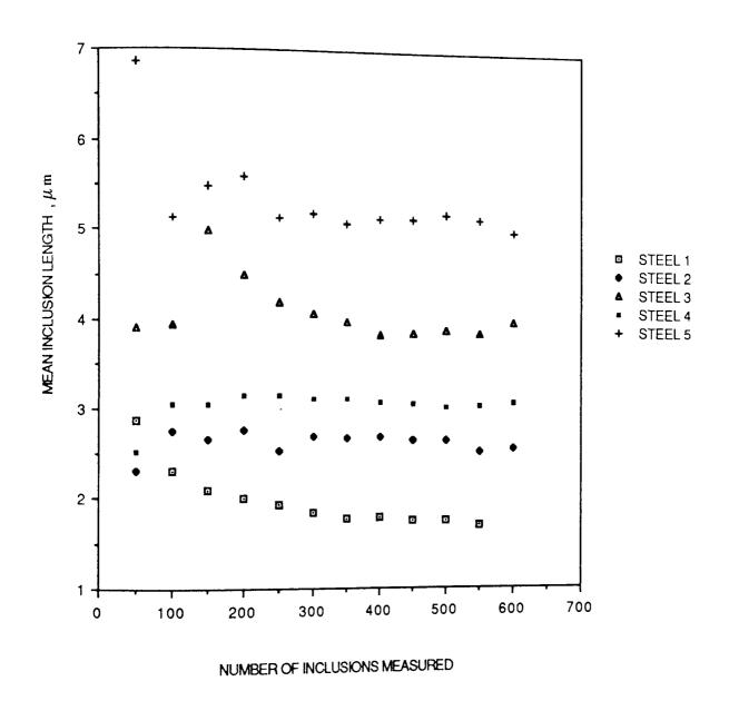
FIGURE 43. MEAN INCLUSION LENGTH VERSUS NUMBER OF INCLUSIONS MEASURED FOR STEELS 1-5.
