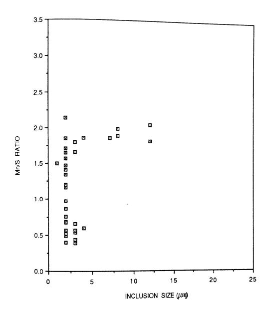
FIGURE 65. Mn/S RATIO FOR THE INCLUSIONS IN STEEL 3.
