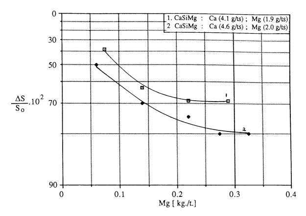
FIGURE 10. Desulphurising by magnesium injection <sup>88</sup>
