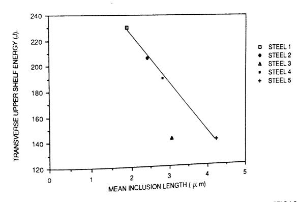
FIGURE 101. TRANSVERSE UPPER SHELF ENERGY VERSUS MEAN INCLUSION LENGTH FOR STEELS 1-5.
