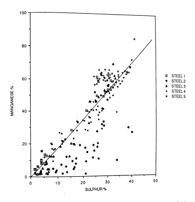
FIGURE 94. MANGANESE VERSUS SULPHUR CONTENT FOR THE INCLUSIONS IN STEELS 1-5.
