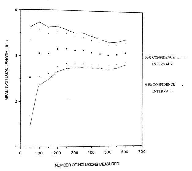
FIGURE 47. MEAN INCLUSION LENGTH VERSUS NUMBER OF INCLUSIONS MEASURED IN STEEL 4.
