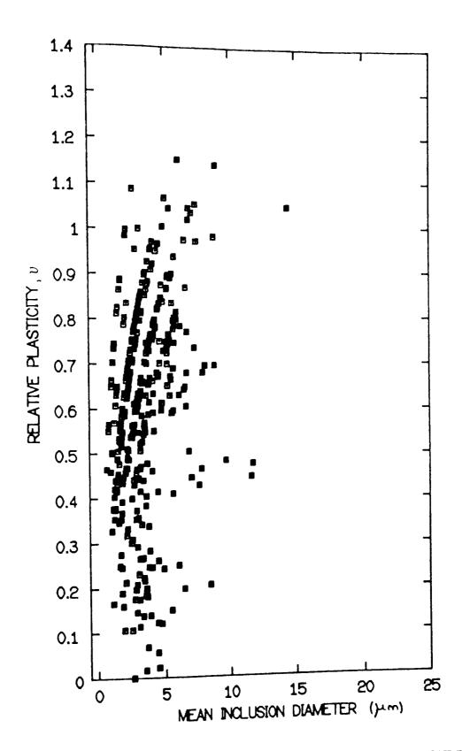
FIGURE 34 RELATIVE PLASTICITY OF THE INCLUSIONS IN THE 0.017% SULPHUR UNTREATED STEEL ROLLED AT 1000°C
