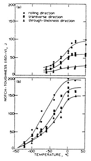
Influence of Ca injection on notch toughness of 50 mm plate of FG 36 steel.
