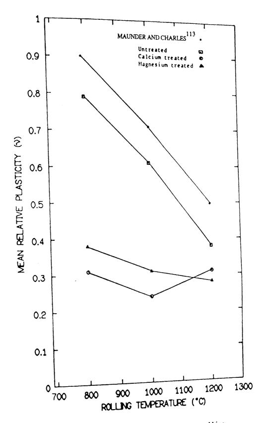
FIGURE 97 Mean relative plasticity versus rolling temperature
