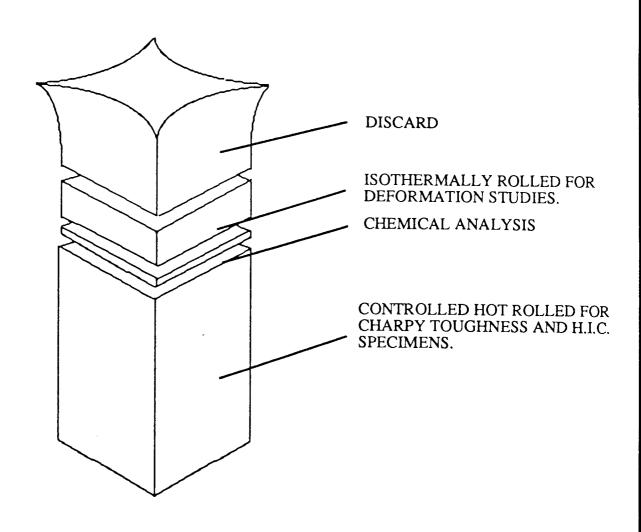
FIGURE 15. Sectioning procedure for the 'as-cast' ingot
