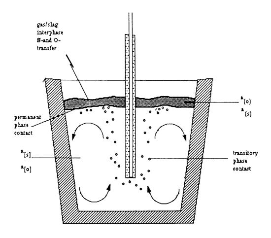
FIGURE 5. Desulphurisation model for ladle injection under top slag 22.
