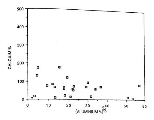
FIGURE 90. CALCIUM VERSUS ALUMINIUM FOR THE INCLUSIONS IN STEEL 2.
