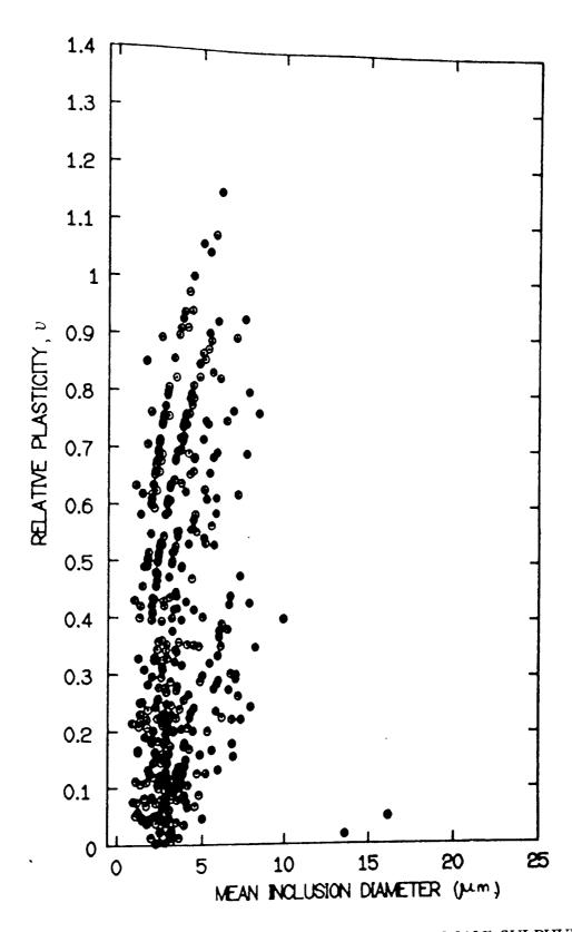
FIGURE 30 RELATIVE PLASTICITY OF THE INCLUSIONS IN THE 0.013% SULPHUR MAGNESIUM TREATED STEEL ROLLED AT 800°C
