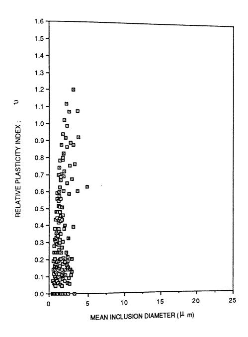
FIGURE 37. RELATIVE PLASTICITY INDEX VERSUS SIZE FOR STEEL 1. (CONTROLLED ROLLED)
