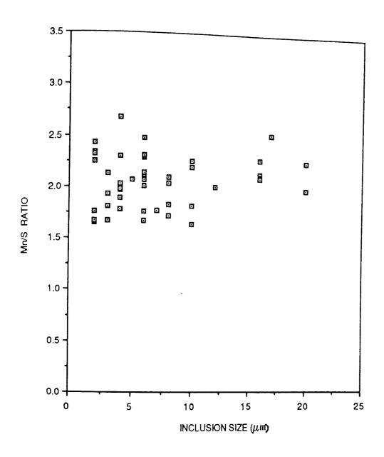
FIGURE 67. Mr/S RATIO VERSUS SIZE FOR THE INCLUSIONS IN STEEL 5.
