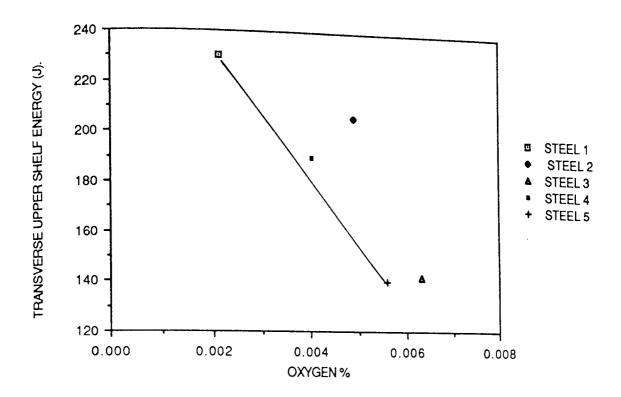
FIGURE 98. TRANSVERSE UPPER SHELF ENERGY VERSUS OXYGEN CONTENT FOR STEELS 1-5.
