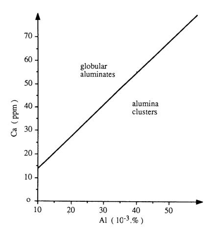
FIGURE 8. Relationship between calcium content and aluminium content in a killed steel to obtain spheroidisation of alumina clusters 73.
