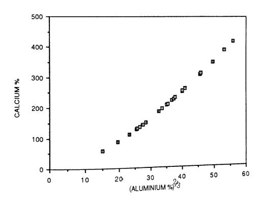
FIGURE 89. CALCIUM VERSUS ALUMINIUM FOR THE INCLUSIONS IN STEEL 3
