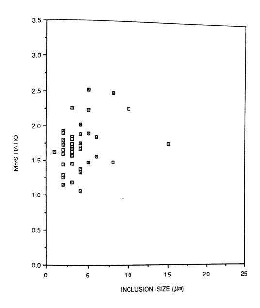
FIGURE 66. Mr/S RATIO VERSUS SIZE FOR THE INCLUSIONS IN STEEL 4.
