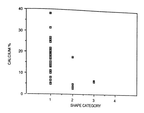
FIGURE 70. INCLUSION SHAPE VERSUS CALCIUM CONTENT FOR STEEL 2.
