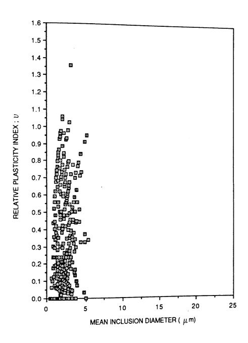
FIGURE 40. RELATIVE PLASTICITY INDEX VERSUS SIZE FOR STEEL 4 (CONTROLLED ROLLED)
