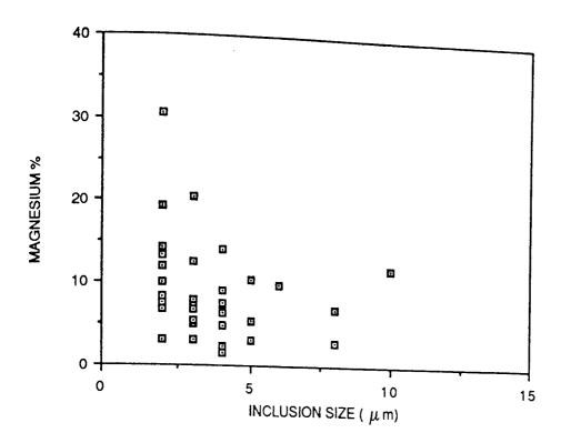
FIGURE 72. INCLUSION SIZE VERSUS MAGNESIUM CONTENT FOR STEEL 4.
