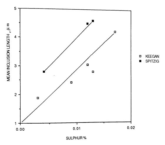
FIGURE 49. MEAN INCLUSION LENGTH VERSUS SULPHUR CONTENT
