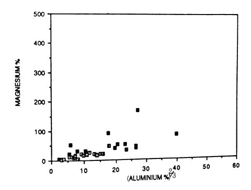
FIGURE 93. MAGNESIUM VERSUS ALUMINIUM CONTENT FOR THE INCLUSIONS IN STEEL 4.
