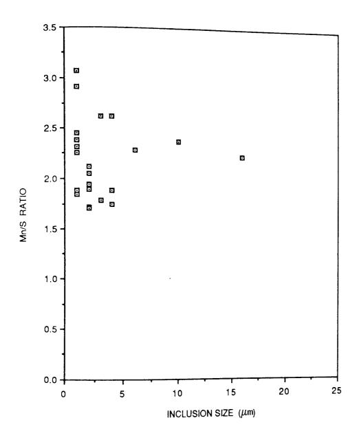
FIGURE 63. Mr/S RATIO VERSUS SIZE FOR THE INCLUSIONS IN STEEL 1.
