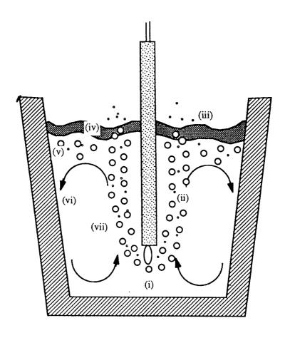
FIGURE 4. Reactor model for ladle injection according to Lehner 48.
