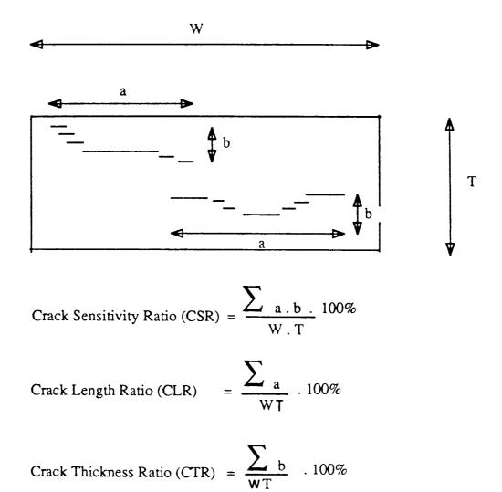
FIGURE 17. Method used for the quantitative evaluation of S.W.C. in metallographic sections.
