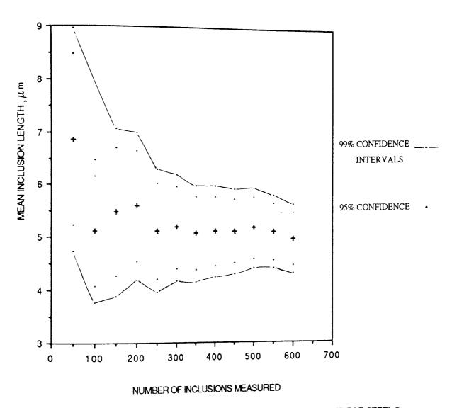
FIGURE 48. MEAN INCLUSION LENGTH VERSUS NUMBER OF INCLUSIONS MEASURED FOR STEEL 5.
