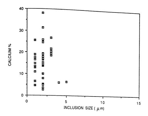
FIGURE 68. INCLUSION SIZE VERSUS CALCIUM CONTENT FOR STEEL 2.
