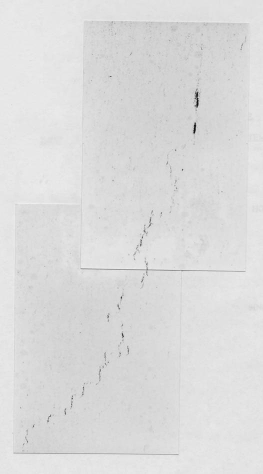
Figure 105. Elongated inclusions associated with hydrogen induced cracking.
