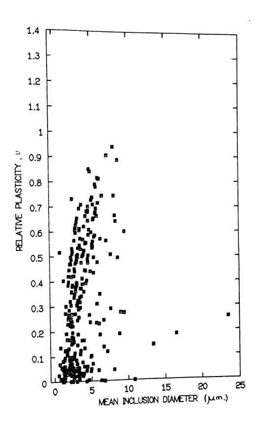
FIGURE 29 RELATIVE PLASTICITY OF THE INCLUSIONS IN THE 0.012% SULPHUR CALCIUM TREATED STEEL ROLLED AT 1200°C
