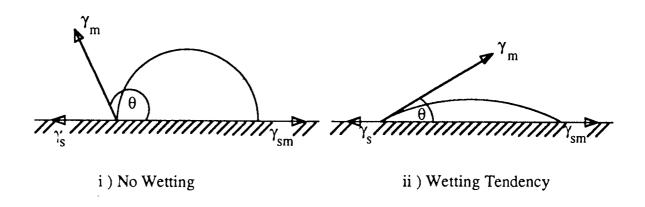
FIGURE 1. Form of a droplet of metal resting on a solid oxide support.<sup>25</sup>.
