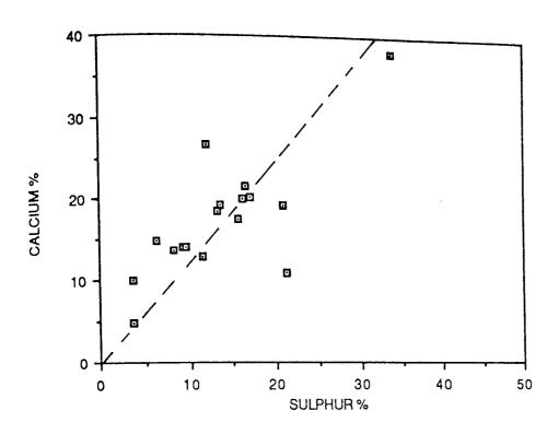
FIGURE 86. CALCIUM VERSUS SULPHUR CONTENT FOR THE INCLUSIONS IN STEEL 2.
