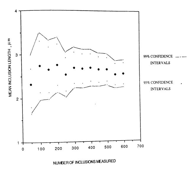
FIGURE 45. MEAN INCLUSION LENGTH VERSUS NUMBER OF INCLUSIONS MEASURED FOR STEEL 2.
