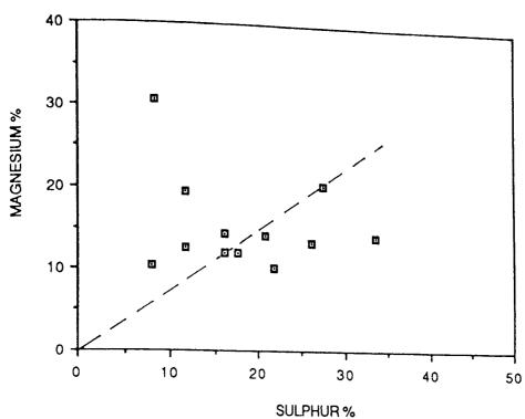
FIGURE 92. MAGNESIUM VERSUS SULPHUR CONTENT FOR THE INCLUSIONS IN STEEL 4
