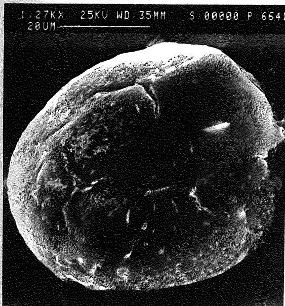
Plate 4.1.7c P(HB-HV) Microsphere (KX1,27) after 23 days incubation in 1.5% pancreatin solution.
