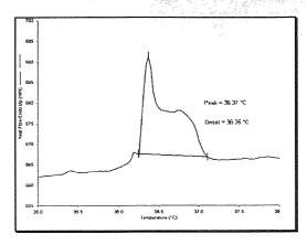
Figure A2.10 – DSC scan for DSPC:Chol, (16:4) liposomes with 1 mg EP incorporated.
