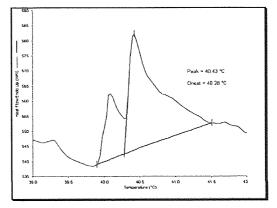
Figure A2.12 – DSC scan for DSPC:Chol, (16:4) liposomes with 1 mg BP incorporated.
