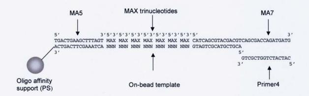
**Figure 4.4:** Schematic representation of the redesigned oligonucleotides in relation to each other. MA7 is longer than MA6 (Figure 4.1) and Primer 4 has a sequence that is not found on the template strand.
