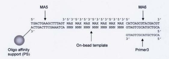
**Figure 4.1:** Schematic representation of the on-bead template showing the hybridisation oligonucleotides (MA5 and MA6) and reverse primer (Primer3). Note that MA5 also serves as the forward primer.
