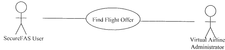
Figure C.13: Use Case Diagram of the SecureFAS Prototype System Find Flight Offer Process
