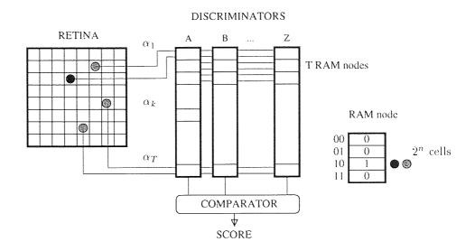
Figure 2.1: The Architecture of the Binary RAMnet.
