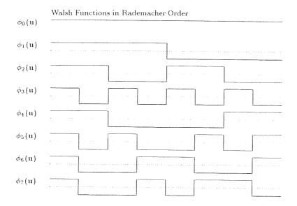
Figure 3.3: Set of Walsh functions  $\{\phi_i\}$  in Rademacher order for n=3. X-axis is  $\mathbf{u}$ , regarded as a single binary number.
