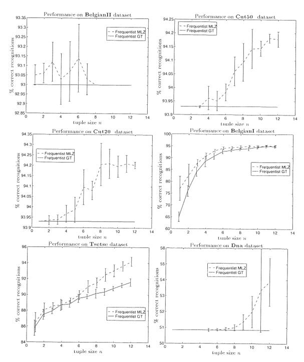
Figure 5.4: Performance of the n-tuple system with Good-Turing estimates (GTE) compared with Maximum Likelihood estimates system (MLZ) with zero tally correction ( $\epsilon = 10^{-150}$ ). The systems comprised of 100 tuples. The error-bars are of size one standard deviation computed for 10 random tuple mappings.
