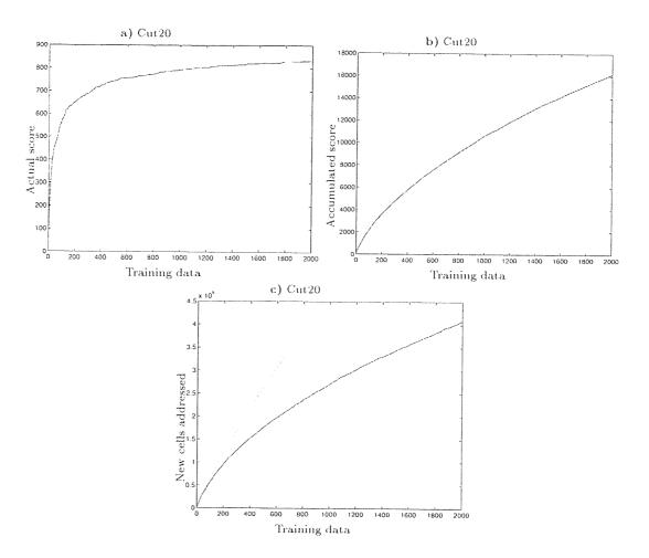
Figure 4.4: a) actual network response to a test pattern u; b) accumulated network response (as though patterns never overlapped on any tuples) and c) the number of new RAM cells addressed as a function of training patterns. Light lines are used to indicate the discriminator associated with the class that generated u, dark lines denote the other class. The training data is sorted by the Hamming distance to the test pattern.
