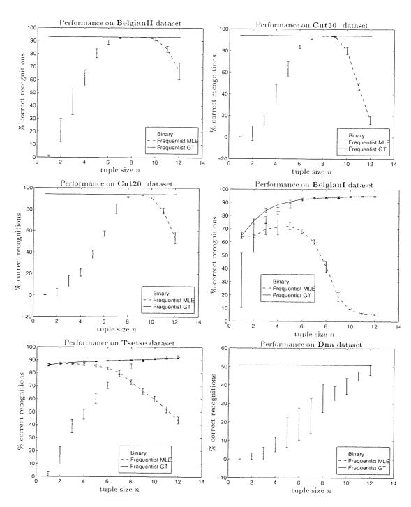
Figure 5.3: The MLE and GTE RAMnet's performance compared to that of binary n-tuple system for various values of tuple size n. All systems comprised of 100 tuples. The error-bars are of size one standard deviation computed for 10 random tuple mappings.
