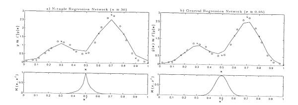
Figure 3.6: a) Performance of the n-tuple regression network with n=30, T=100 on a simple regression problem. The lower graph shows the effective tuple kernel K(x,x') centered on a bit string corresponding to x=0.5. Training and test data is shown by circles and crosses respectively. b) Performance of the Specht's regression network with a Gaussian kernel for parameter  $\sigma=0.05$  on the same data. The shape of the kernel is shown on the lower plot.
