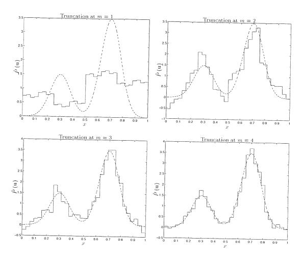
Figure 3.4: Truncated Rademacher-Walsh approximation to a Gaussian mixture probability density function. Approximation  $\hat{P}(\mathbf{u})$  improves with increasing m. The coefficients were estimated from a sample of size  $10^5$  and the approximation calculated according to the equation 3.18. The real valued input x was thermometer encoded into a bit-string  $\mathbf{u}$ .
