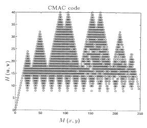
Figure 2.2: Hamming distance  $H(\mathbf{u}, \mathbf{v})$  between two CMAC/Gray-transformed integers vs. their Manhattan distance M(x, y), for  $3 \times 10^4$  randomly chosen pairs of integers. K = 8 and a = 5. The relationship is linear for Hamming distances up to K, and the transformed distance is bounded below by K for greater Hamming distances.
