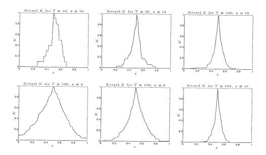
Figure 3.2: Dependence of the effective tuple kernel K on the tuple size and number. The panels show the kernel shapes (solid line) for T=10,30,100 and n=4,8,16. The dotted line indicates the analytical approximation according to equation 3.16. Real numbers  $0 \le x \le 1$  were thermometer encoded with resolution 256 bits yielding a test set  $\{\mathbf{v}^i\}$   $1 \le i \le 256$ . The RAMnet was trained on a bit string  $\mathbf{u}$  corresponding to x=0.5.
