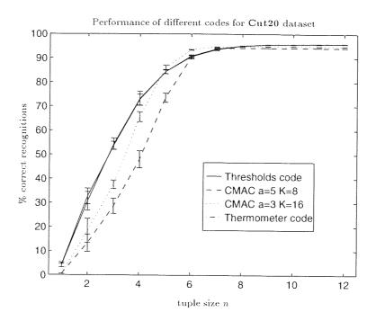
Figure 4.1: RAMnet's performance on Cut20 as a function of tuple size n for CMAC code with a=5, K=8 and a=3, K=16, Thermometer code with resolution 100 bits and Random Thresholds code with 100 thresholds. The error bars of size  $\pm$  1 standard deviation are centred around the mean performance measured for 10 runs. The Random Thresholds code and Thermometer code curves overlap.
