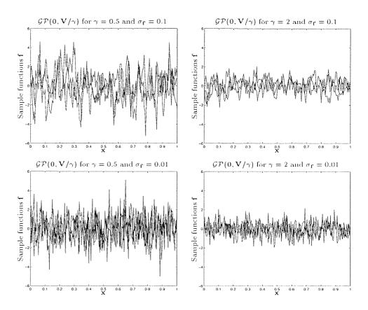
Figure 6.4: Samples from the Gaussian process prior  $\mathcal{GP}(\mathbf{0}, \mathbf{V}/\gamma)$  with the covariance matrix of the form  $V_{rx'} = \exp\left(-\gamma \frac{|x-x'|}{\sigma_t^2}\right)$  for various choices of the parameters  $\gamma$  and  $\sigma_{\mathbf{f}}$ .
