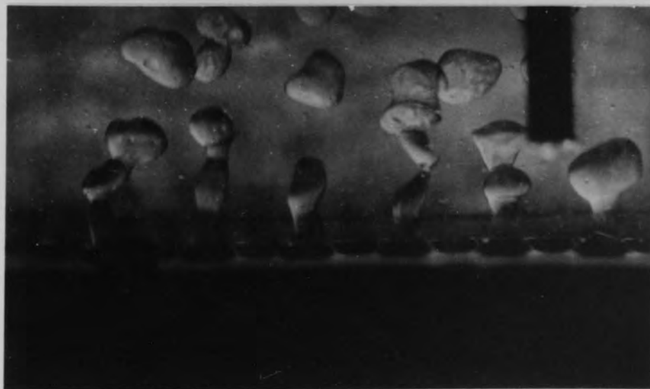
Fig 8.2-28 Relationship between drop shapes, dispersed phase throughputs and Reynolds number - Plate † 4.763 mm i.d. hole size.
