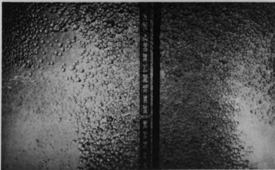
Fig. 8.1-3 Droplet dispersion between plates 2 and 3 1.588 mm i.d. hole size.
