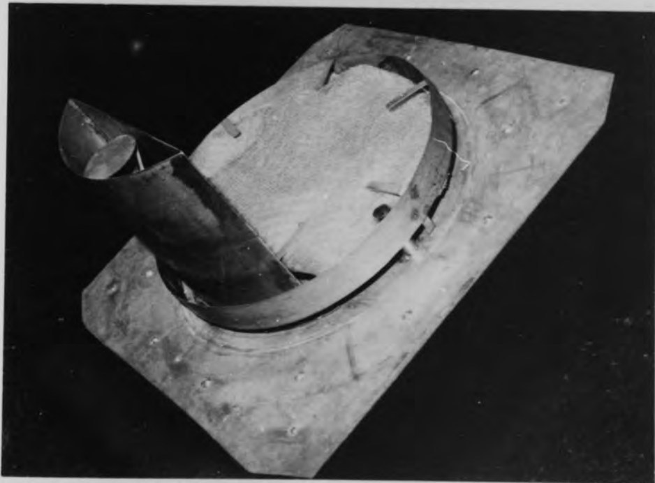
Fig. 7.2-7 Top Cover Detail Knitmesh pad in position for coalescence of outlet dispersion. First downcomer continuous phase input.
