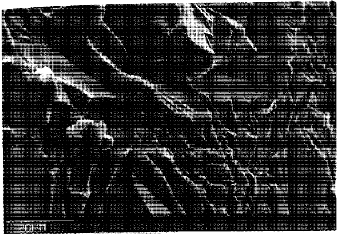
Plate 10.6 Crust surface of a particle dried at an air velocity of 3.0 \text{ ms}^{-1} ( C_o = 15 \text{ wt.}\% , T_g = 22^\circ\text{C} )
