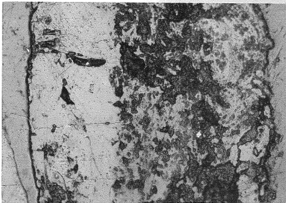
Figure 51: Cross-section of Lead-free Deposit showing High Degree of Porosity
