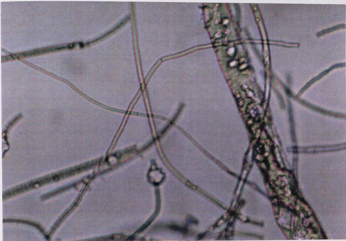
Plate 5.2. (x25) 1 Hour Degradation. L.Pec.9.; PHB(FM)IP Blended With 9% Low Molecular Weight Pectin, Illustrating The Cavities Of Degraded Pectin In The Large And Medium Sized Fibres And The Smooth Small Diameter Fibres.
