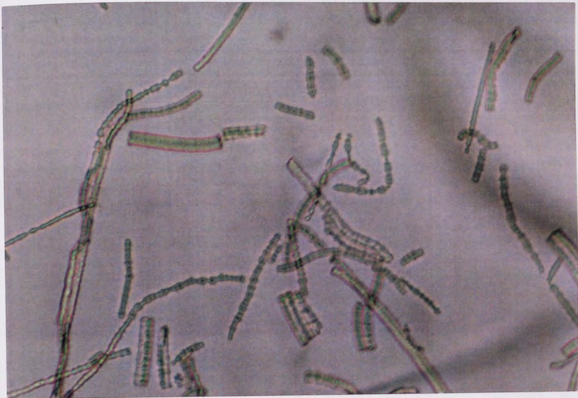
Plate 5.58. (x25) 1 Hour Degradation. PHB/5V.; PHB(FM)IP Blended With 5% Poly( \beta -hydroxyvalerate) After 1 Hours Degradation, Illustrating The Irregular 'Banded' Small Diameter Fibres.
