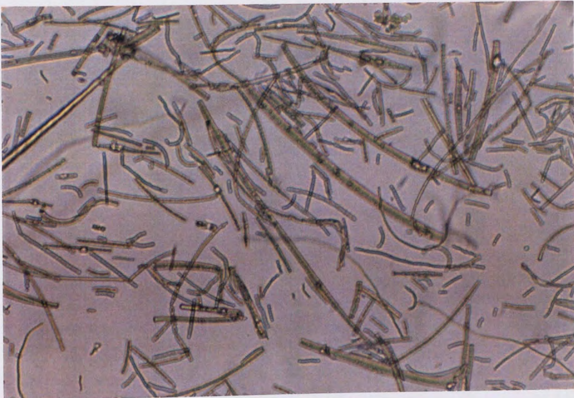
Plate 5.11. (x10) 7 Hours Degradation. L.Pec.15.; Fragmentation Of Matrix After 7 Hours Degradation.
