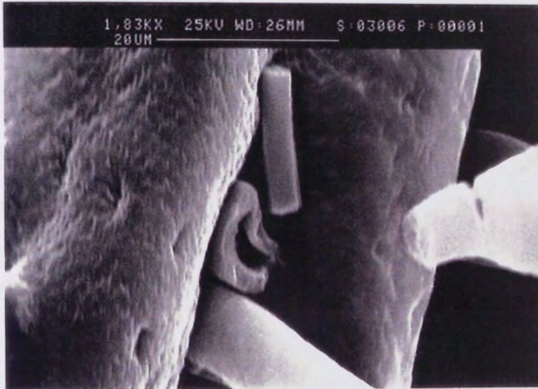
Plate 4.35. (x1.83K) 4 Days Degradation. PHB(FM)IP; Heavily Pitted And Porous Large Diameter Fibre With A Fragmented Smaller Diameter Fibre Revealing Its Hollow Nature.
