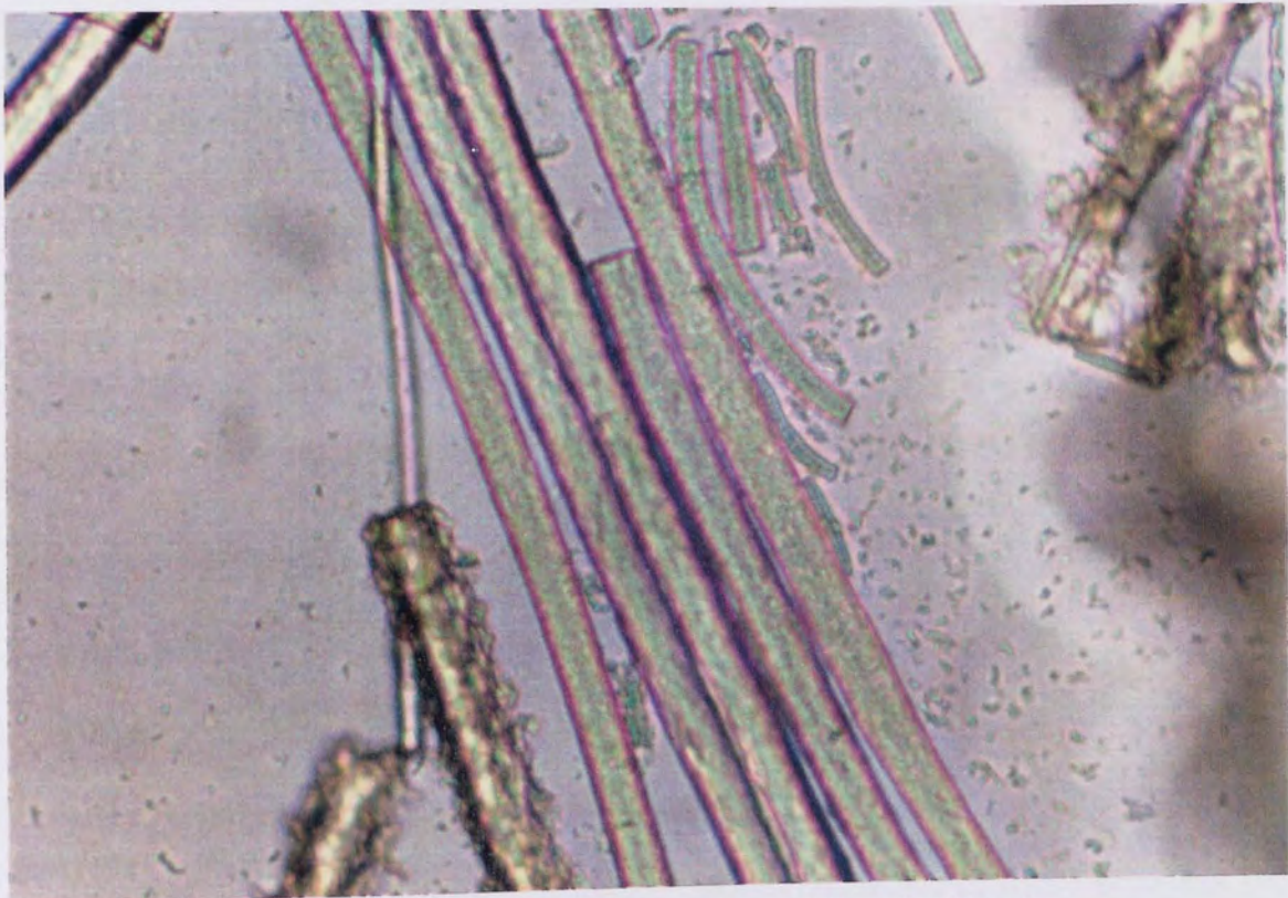
Plate 4.10. (x10) 2.29 Days Degradation (2 Days & 7 Hours). PHB(FM)TG; Fibre Specific Surface Erosion And A Proportion Of Unaffected, Comparatively Smooth Fibres.
