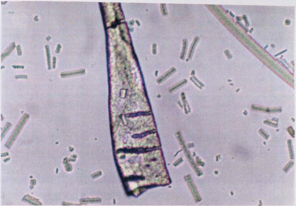
Plate 4.29. (x25) 4 Days Degradation. PHB(FM)IP; Fracturing And Erosion In A Large Diameter Fibre Fragment, Fractures Appear 'Eaten Away'.
