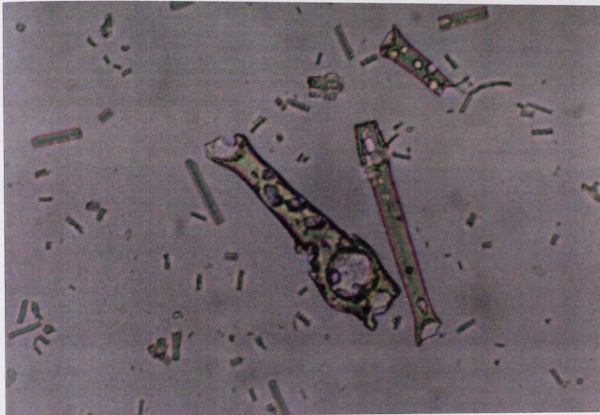
Plate 5.6. (x15) 5 Days Degradation. L.Pec.9.; Large And Medium Diameter Fibres Exhibiting 'Pectin Cavities' And Irregularities.
