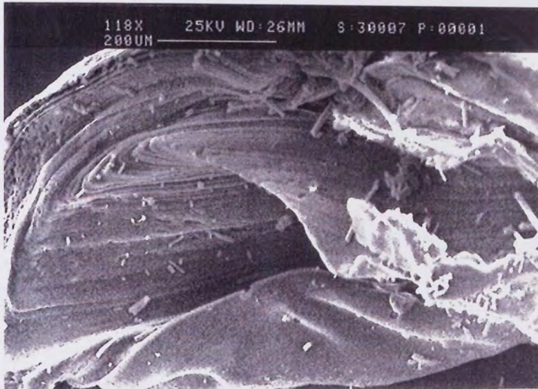
Plate 4.43. (x118) 33 Days Degradation. PHB(FM)IP; Section Of Melt Compressed PHB Mass, Illustrating Its Formation From The Collapsed PHB(FM)IP.
