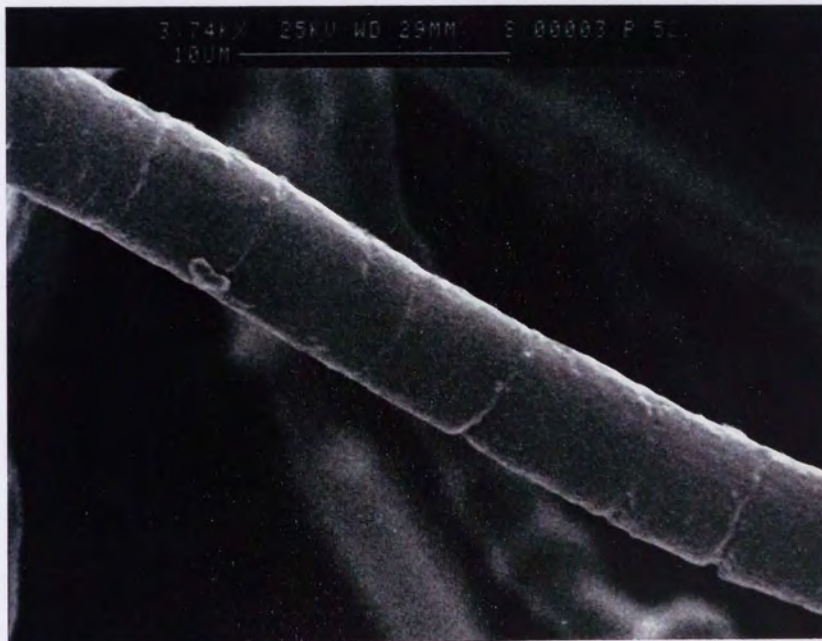
Plate 3.17. (x3.74K) SA-30.; PHB(FM)IP Blended With 30% Sodium Alginate Illustrating A Comparatively Smooth Fibre With Indentations.
