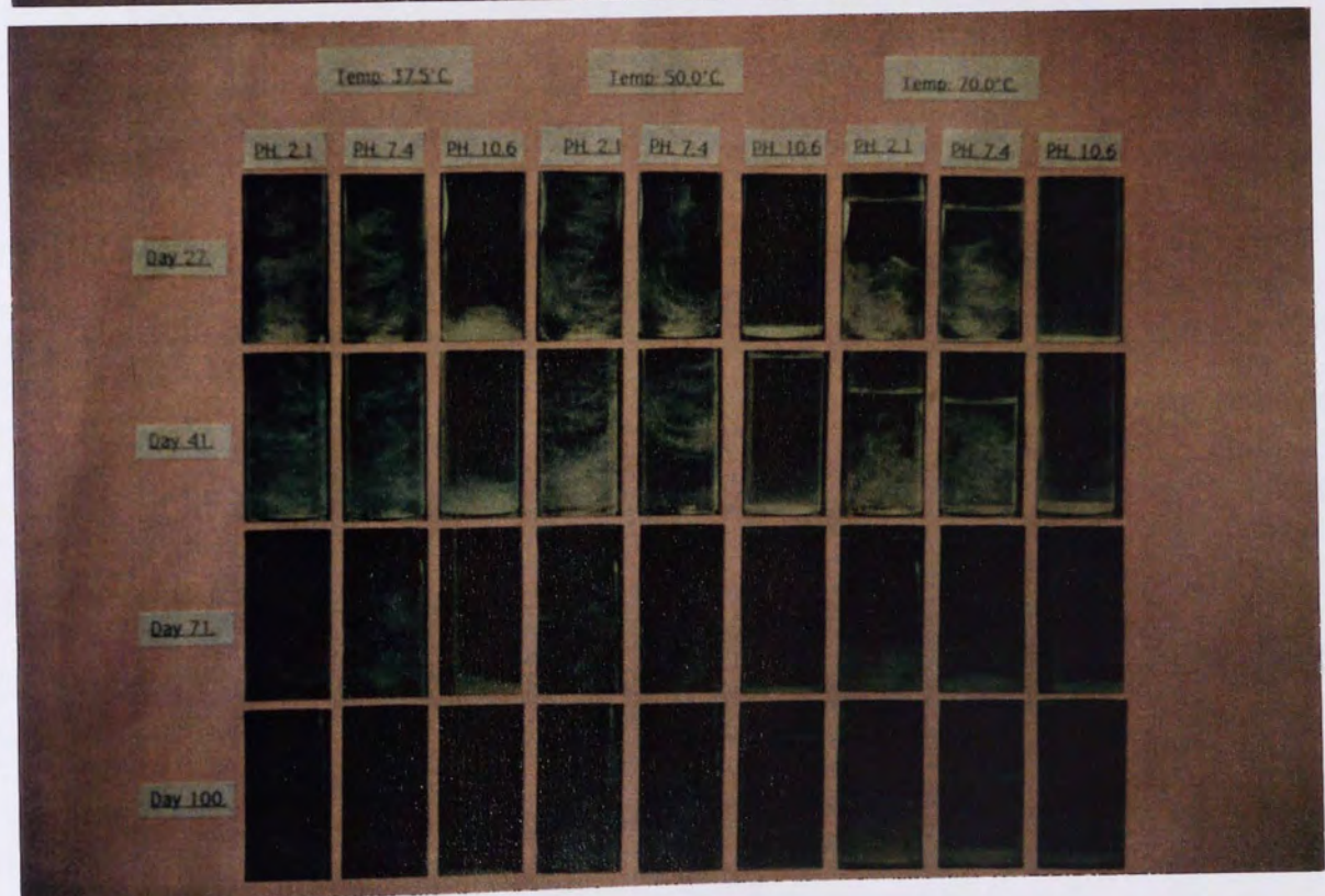
Plate 3.28. Photographic Record Of Qualitative Degradation Of PHB(FM)TG With Varying Temperature And Buffer Conditions.
