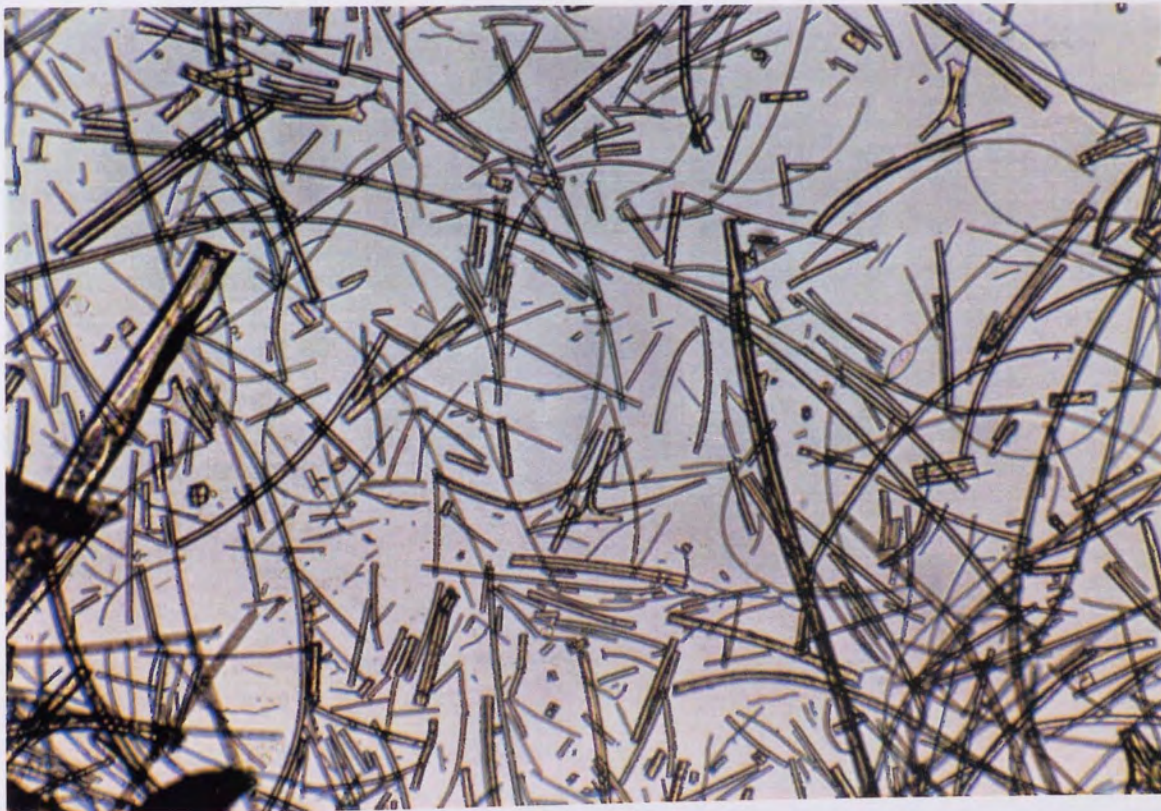
Plate 4.8. (x10) 1 Day Degradation. PHB(FM)TG; Hollow Regions In The Smaller Diameter Fibres And Bubble In The Large Diameter Fibre.
