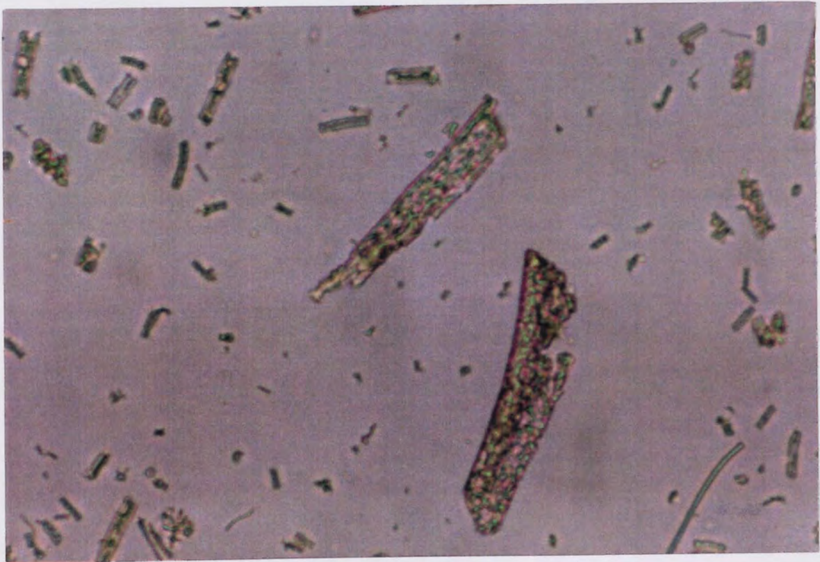
Plate 5.23. (x25) 7 Days Degradation. L.Pec.25.E.; A Similar Degree Of Fragmentation To L.Pec.25.S. In Plate 5.22 But With More Irregularities And Pectin Cavities.
