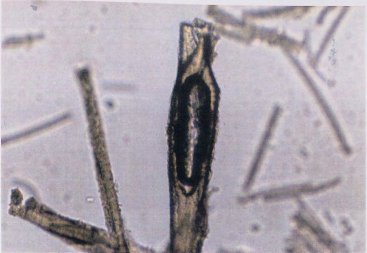
Plate 4.11. (x15) 2.29 Days Degradation (2 Days & 7 Hours). PHB(FM)TG; Hollow Cavity With Bubble.
