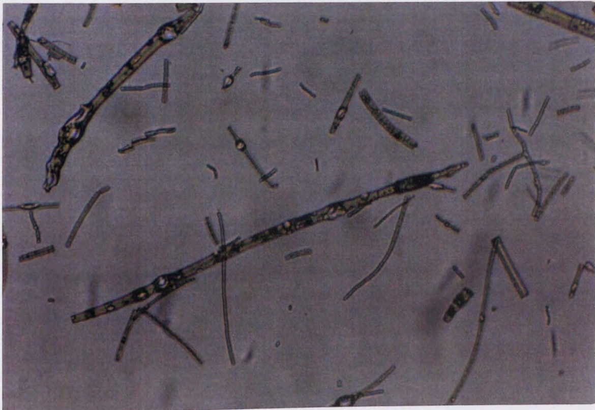
Plate 5.3. (x15) 3 Hours Degradation. L.Pec.9.; Matrix And Fibre Fragmentation.
