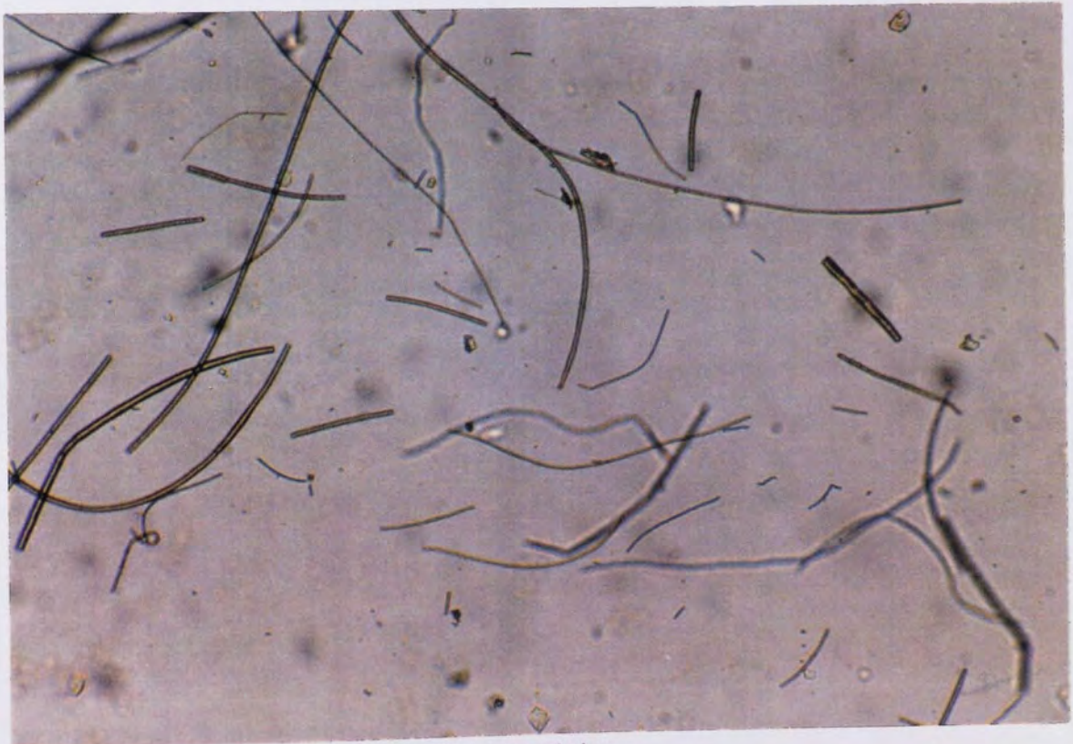
Plate 4.2. (x10) 1 Hour Degradation. PHB(FM)TG; Illustrating The Comparatively Small Degree Of Fragmentation In The Initial Degradation Stage.
