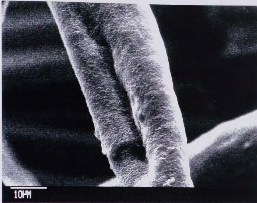
Plate 3.3. (x2.00K) PHB(FM)TG; Forking Of Two Fibres.
