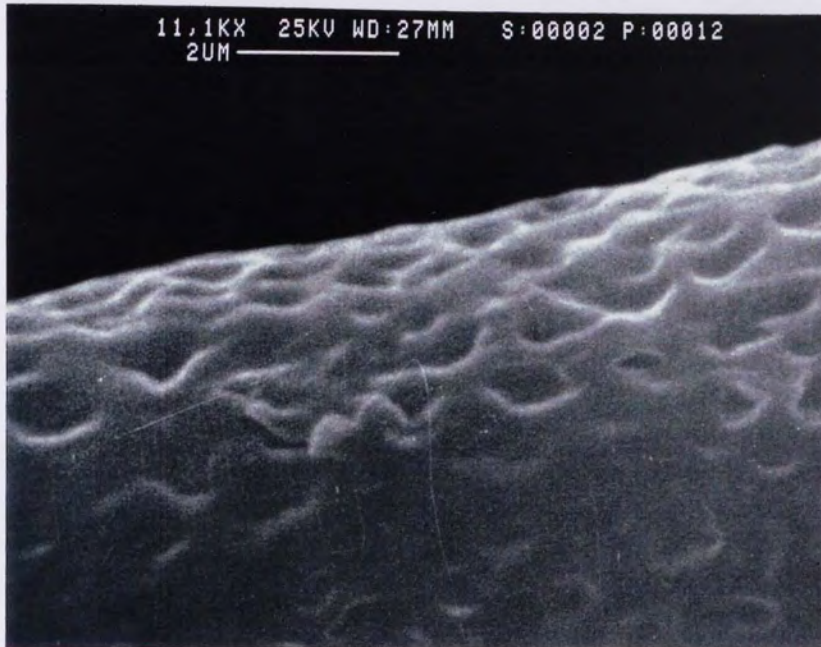
Plate 3.12. (x11.2K) PHB(FM) Produced From Methylene Chloride Extraction, Illustrating The Heavily Porous Nature.
