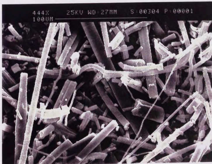
Plate 5.41. (x444K) 1 Day Degradation. L.Pec.25.S.; Fragmentation Of The Mainly Small Diameter Fibres Readily Occurred After 1 Days Degradation.
