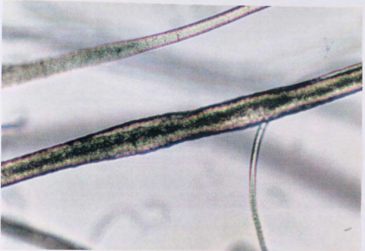
Plate 3.14. (x25) PHB(FM) Produced From Methylene Chloride Extraction, Illustrating A 'Mosaic' Appearance In The Larger Diameter Fibres.
