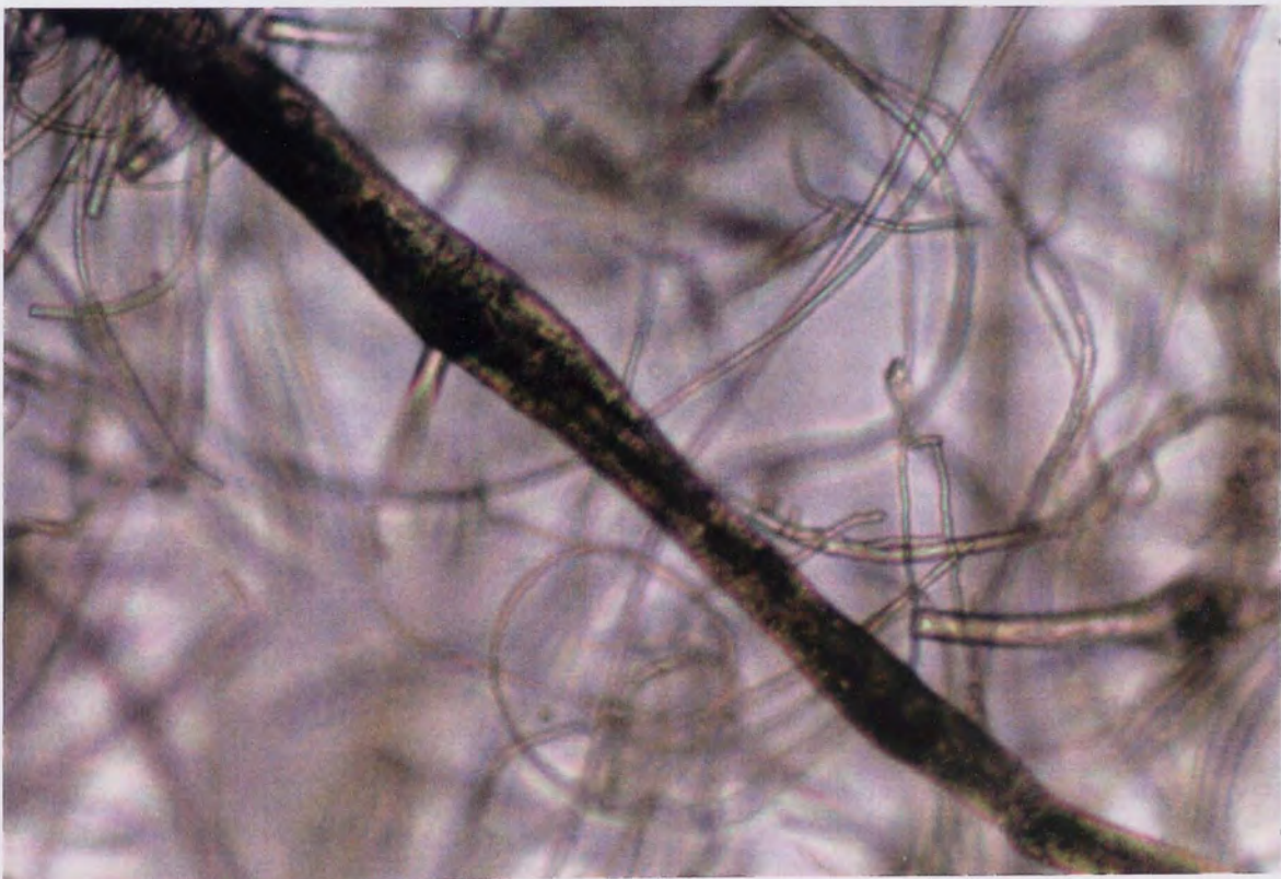
Plate 5.9. (x15) 3 Hours Degradation. L.Pec.15.; Little Matrix Collapse After 3 Hours Degradation, Heavily Pectin Loaded Large Diameter Fibre.
