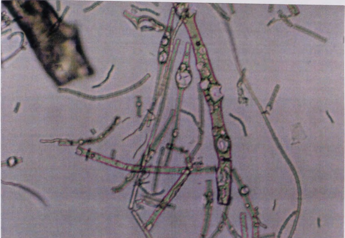
Plate 5.4. (x25) 1 Day Degradation. L.Pec.9.; Fibre Fragmentation And Irregularities, 'Pectin Cavities'.
