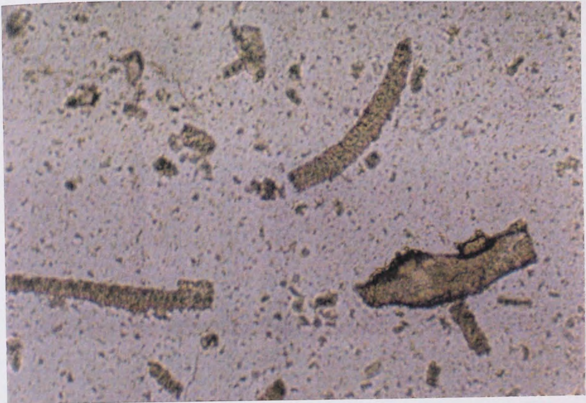
Plate 5.60. (x25) 7 Days Degradation. PHB/5V.; Large Degree Of Fragmentation And To Fibre Fragments With Some Erosion Observed.
