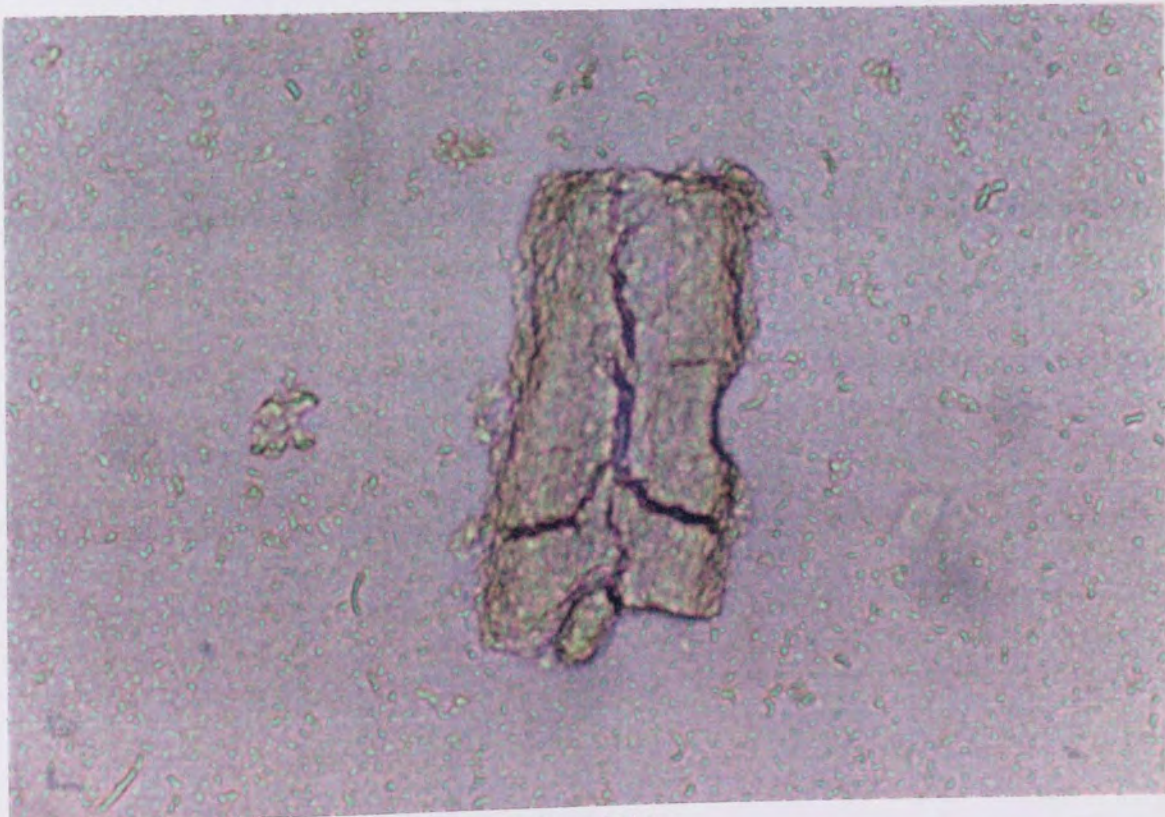
Plate 4.16. (x25) 7 Days Degradation. PHB(FM)TG; Fibre Fragment With Multiple Fragmentation.
