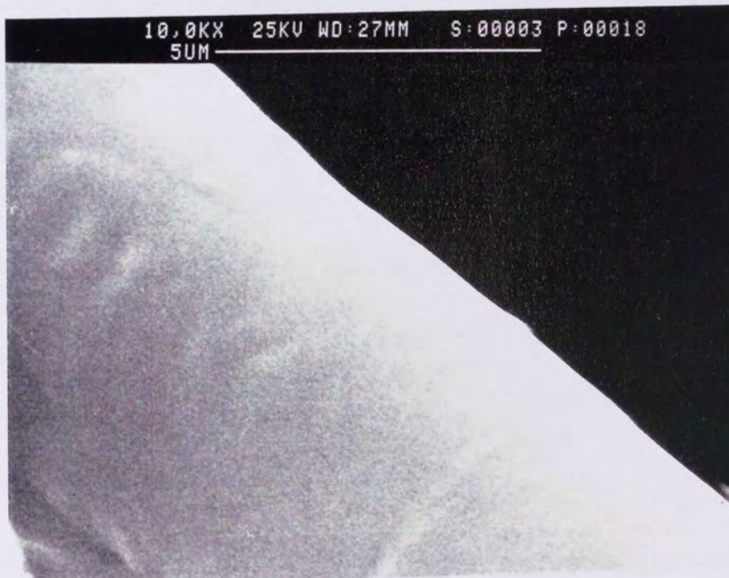
Plate 3.4. (x10.4K) PHB(FM) Produced From Chloroform/Methylene Chloride Extraction, Illustrating A Smooth Fibre.
