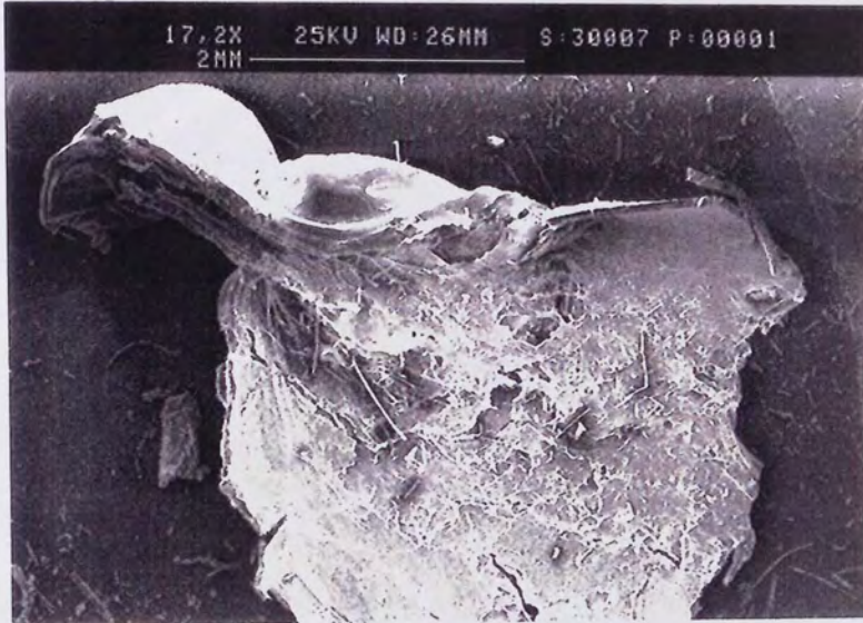
Plate 4.41. (x17.2) 33 Days Degradation. PHB(FM)IP; Residual Melt Compressed PHB Mass From The Phial Base.
