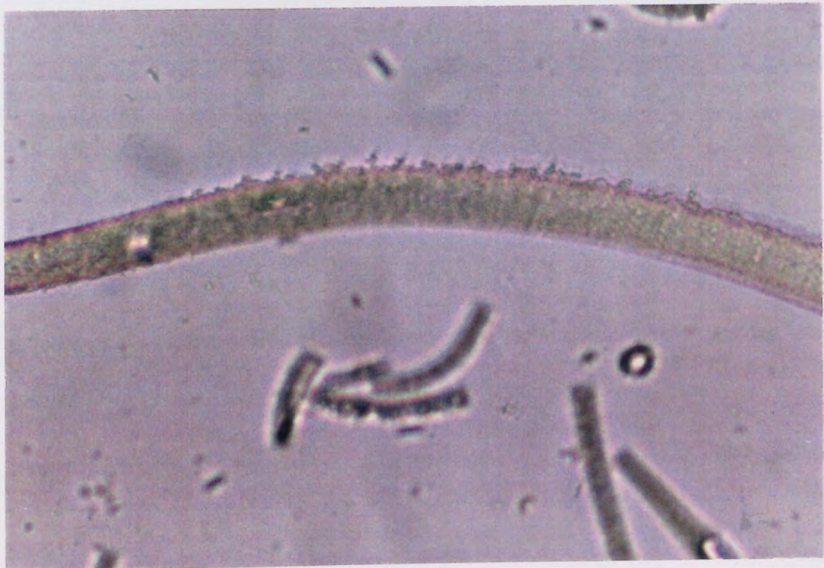
Plate 5.27. (x25) 4 Days Degradation. H.Pec.10.; A Proportion Of Large Diameter Fibres Maintained Integrity But Still Exhibited Surface Erosion.
