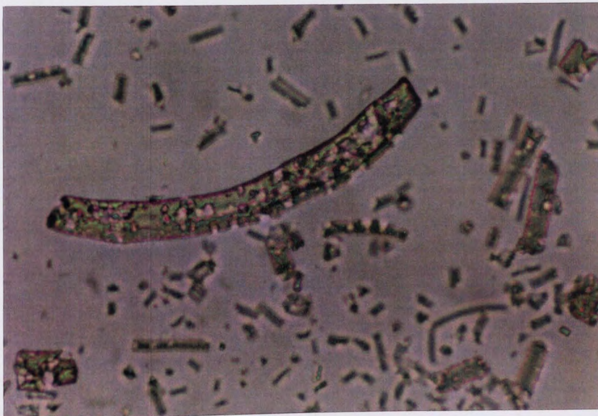
Plate 5.7. (x25) 7 Days Degradation. L.Pec.9.; Readily Noticeable Pectin Cavities In A Large Diameter Fibre.
