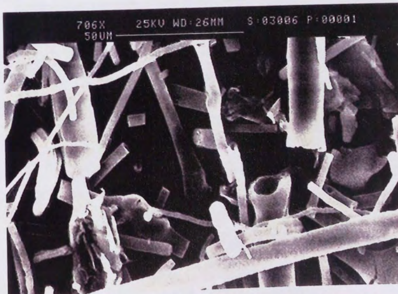
Plate 4.36. (x706) 4 Days Degradation. PHB(FM)IP; Collapsed Matrix And A Fibre Showing The Fragmentation At A Hollow Region Caused By The Release Of A Bubble.
