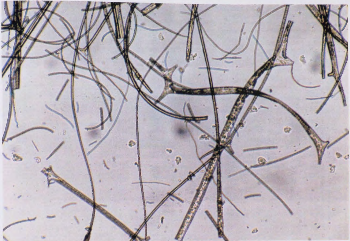
Plate 4.5. (x10) 3 Hours Degradation. PHB(FM)TG; Fragmentation And Gradual Collapse Of The Matrix.
