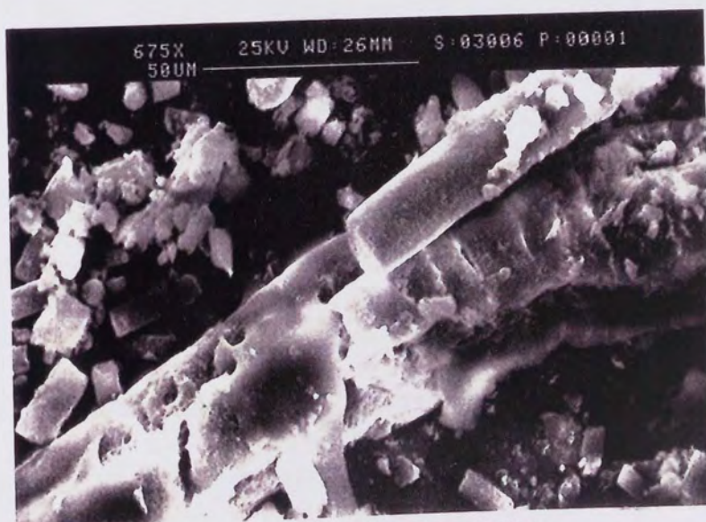
Plate 4.38. (x670) 7 Days Degradation. PHB(FM)IP; Pitted Large Diameter Fibre And Particulate Matter.
