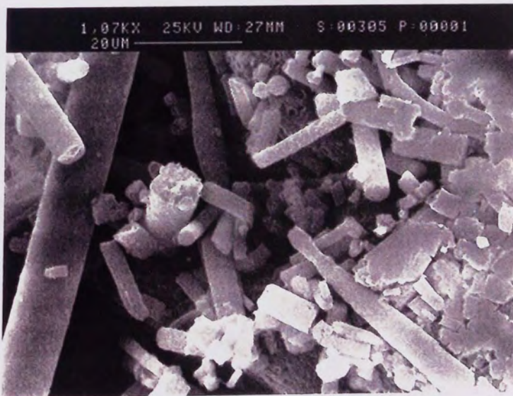
Plate 5.43. (x1.07K) 4 Days Degradation. L.Pec.25.S.; Fibre Fragments And Mat Of Particulate Matter.
