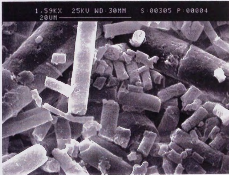
Plate 5.42. (x1.59K) 4 Days Degradation. L.Pec.25.S.; Small Fibre Fragments And Comparatively Intact Large Diameter Fibres.
