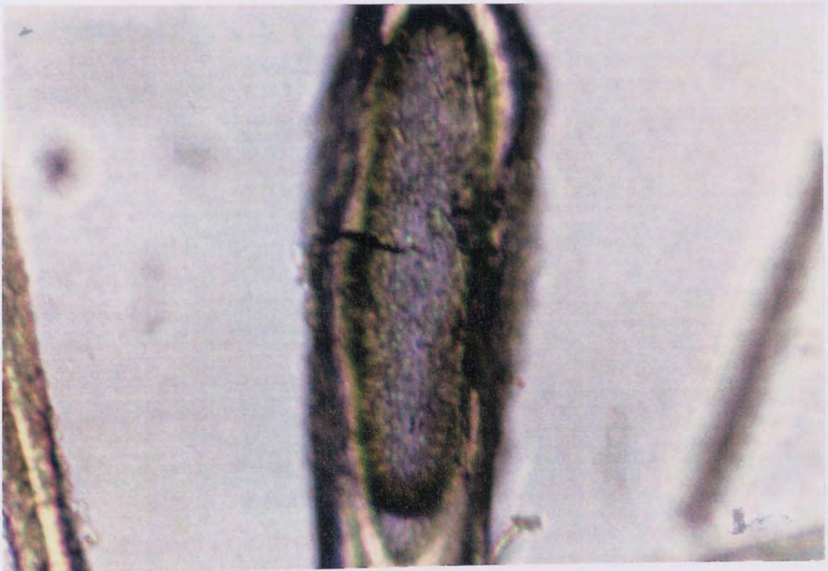
Plate 4.12. (x25) 2.29 Days Degradation (2 Days & 7 Hours). PHB(FM)TG; Hollow Cavity With Fracture And Absence Of Bubble.
