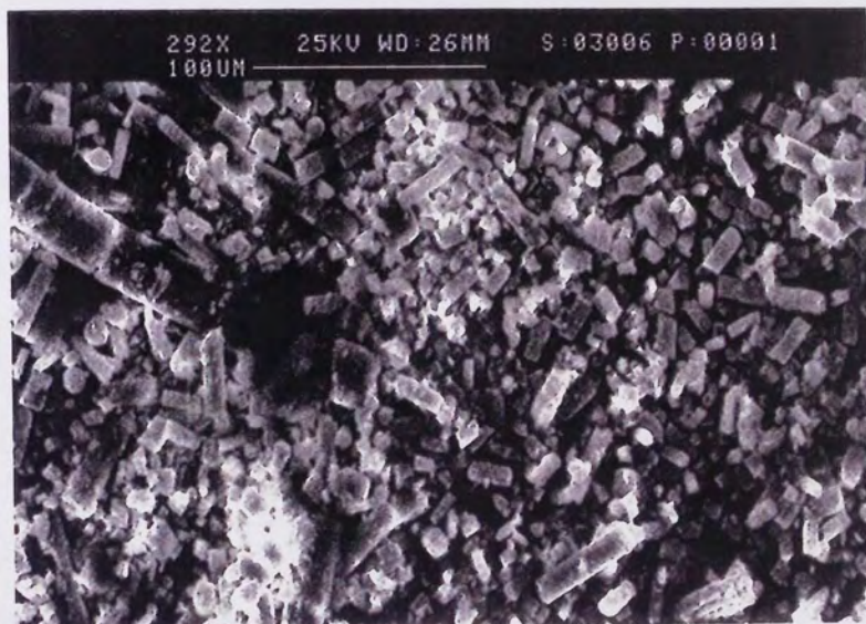
Plate 4.37. (x292) 7 Days Degradation. PHB(FM)IP; Dense Mass Of Small Fibre Fragments And Particulate Matter.
