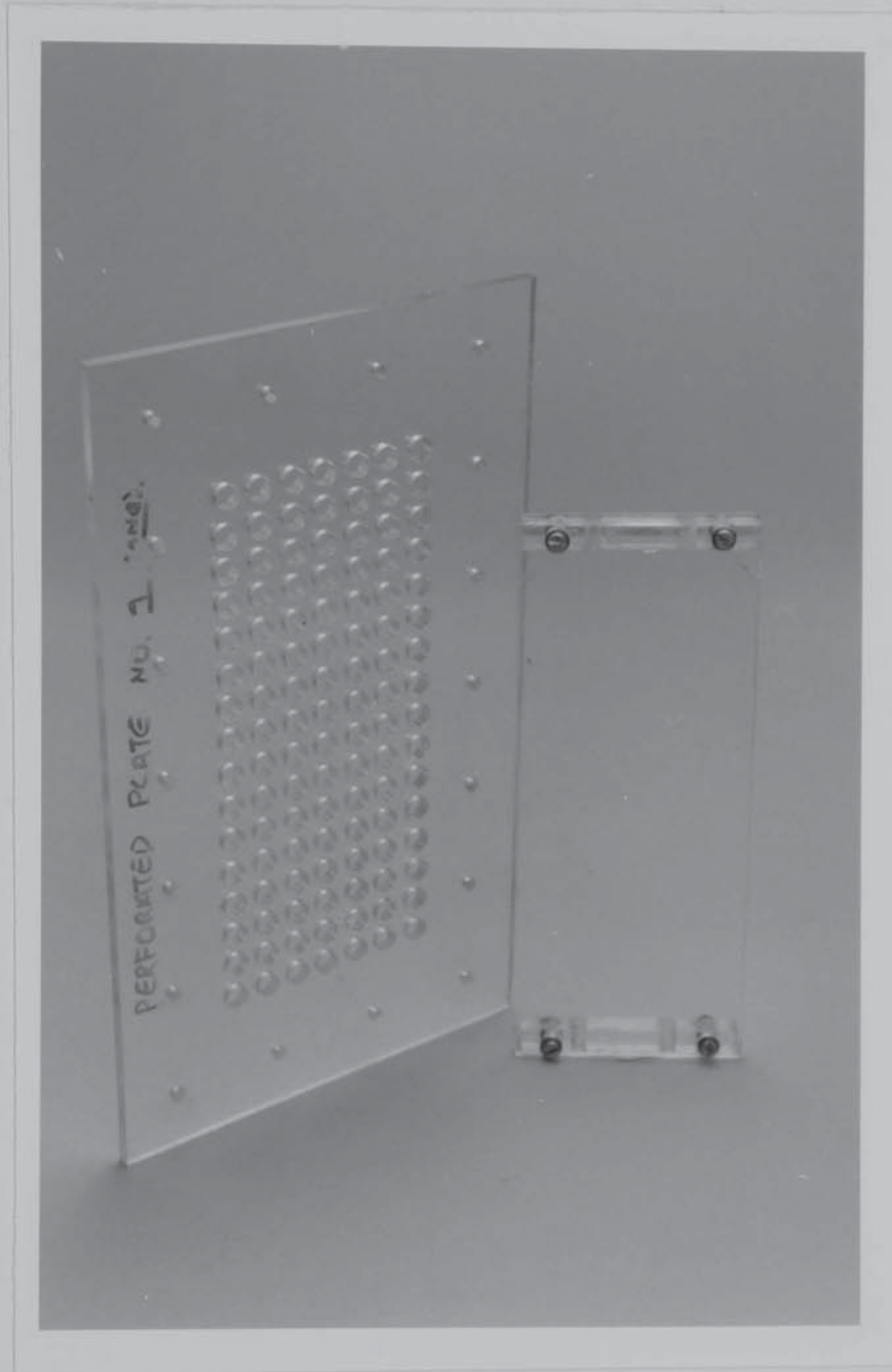
Plate 7.2. Duct Closures (10 cm duct height).
