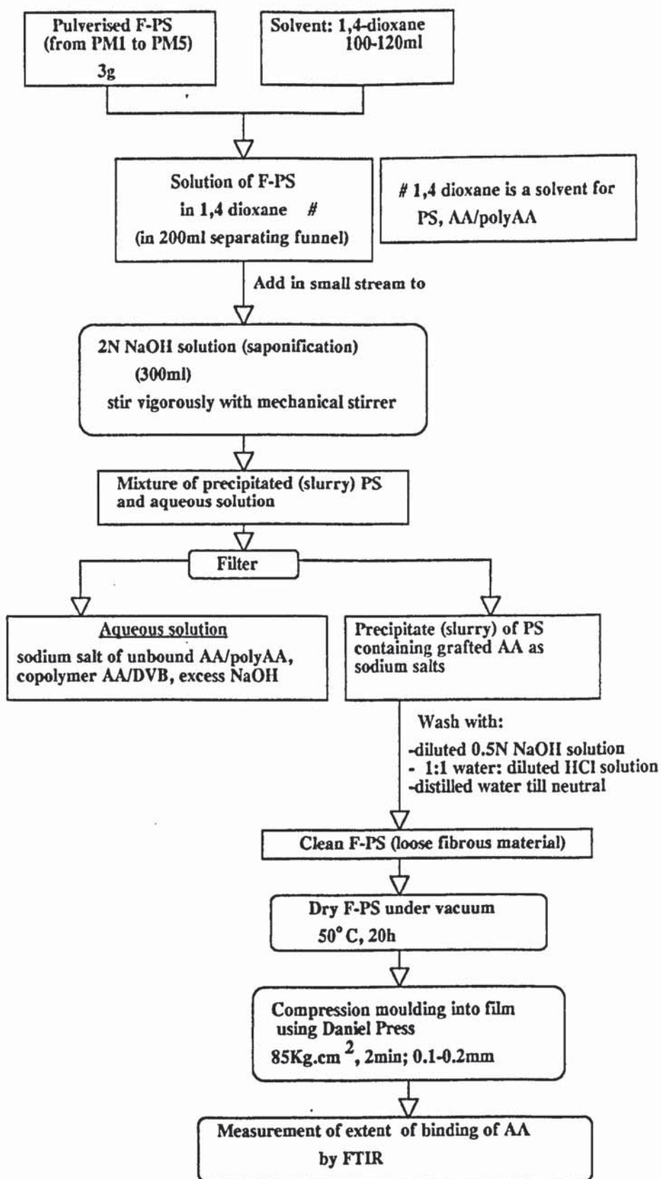
Scheme 3.3: Separation of unbound AA/polyAA from F-PS and determination of concentration of grafted AA to PS by FTIR spectroscopy
