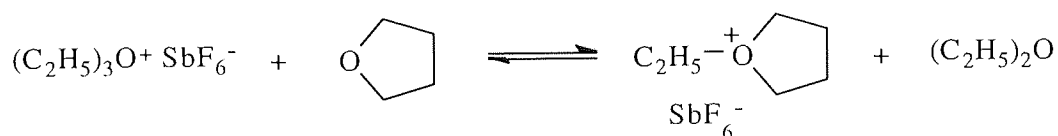
Figure 1.3.7. Initiation of THF with trialkyloxonium salt
