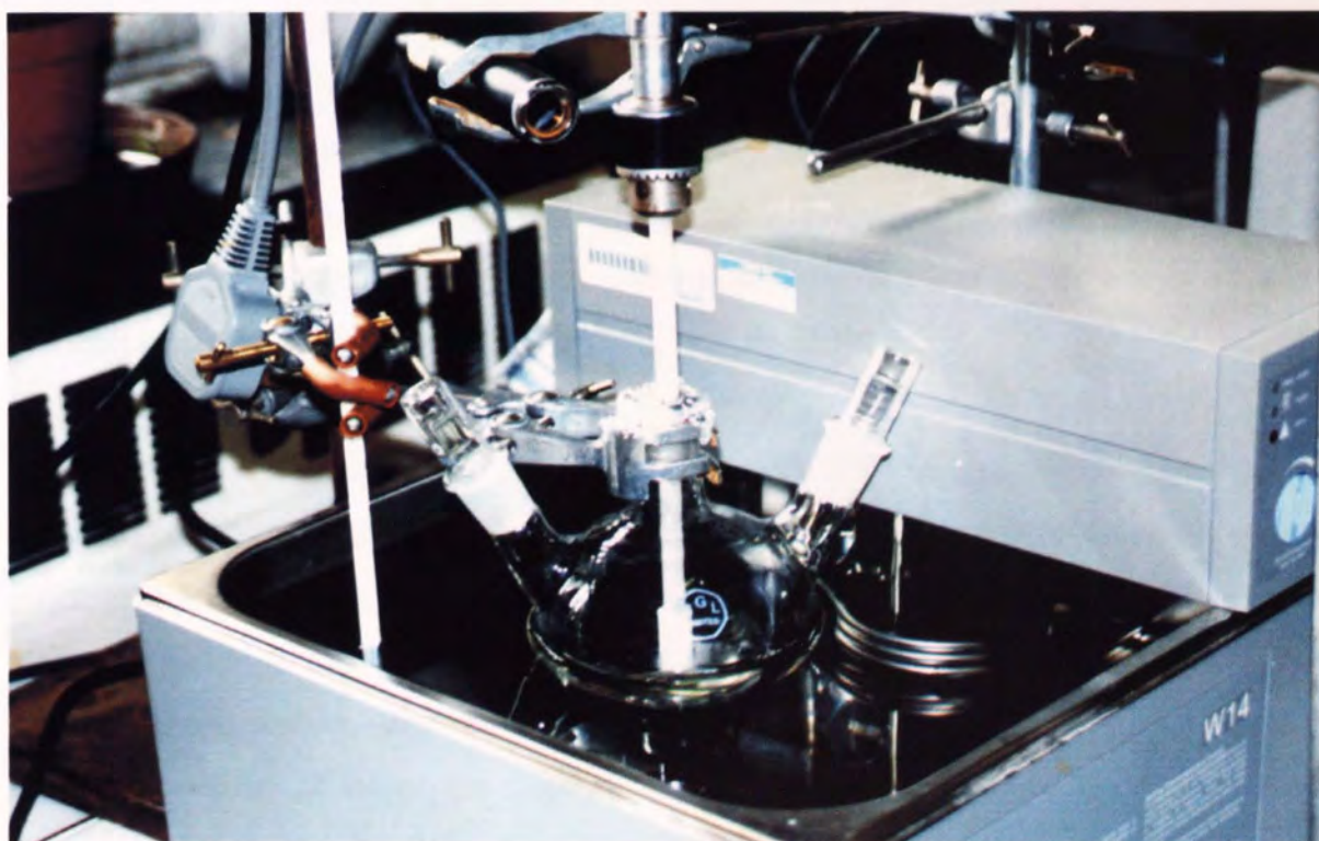
Figure 7.1. The apparatus used to perform stirred-batch reactions.
