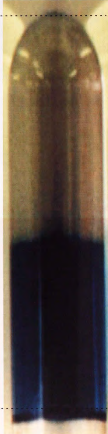
Figure 5.11e. A comparison of the position of blue dextran with the corresponding lactose monohydrate density gradient after centrifugation at 13 000 r.p.m. (26 122 g max) for 180 minutes, at 40°C.
