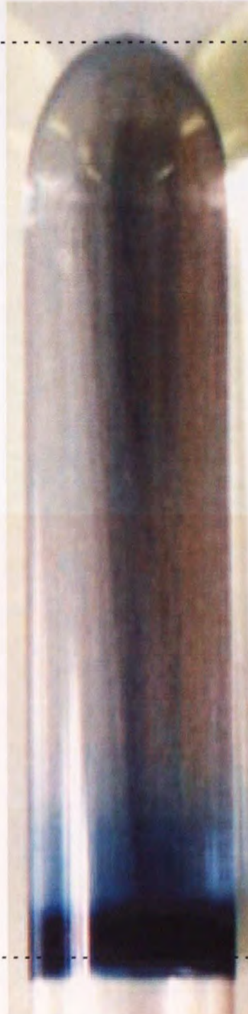
Figure 5.11c. A comparison of the position of blue dextran with the corresponding lactose monohydrate density gradient after centrifugation at 13 000 r.p.m. (26 122 g max) for 60 minutes, at 40°C.
