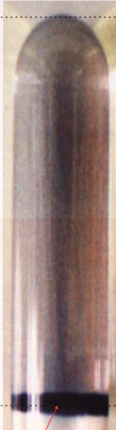
Figure 5.11a. A comparison of the position of blue dextran with the corresponding lactose monohydrate density gradient after centrifugation at 13 000 r.p.m. (26 122 g max) for 0 minutes, at 40°C.
