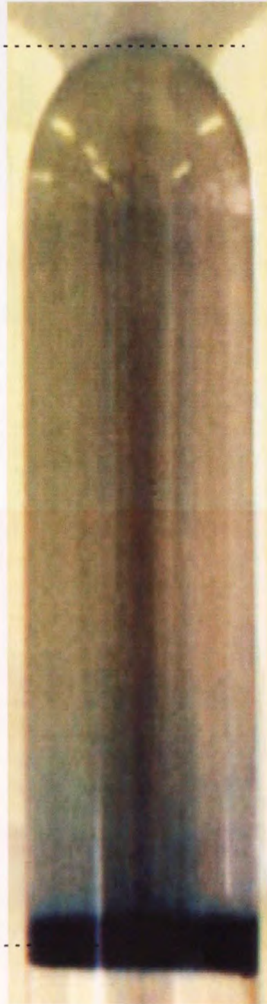
Figure 5.11b. A comparison of the position of blue dextran with the corresponding lactose monohydrate density gradient after centrifugation at 13 000 r.p.m. (26 122 g max) for 30 minutes, at 40°C.
